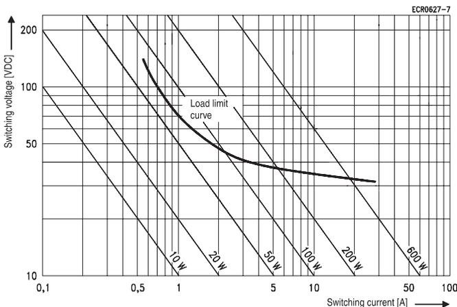
Max. DC load breaking curve: safe shutdown, no stationary arc.
