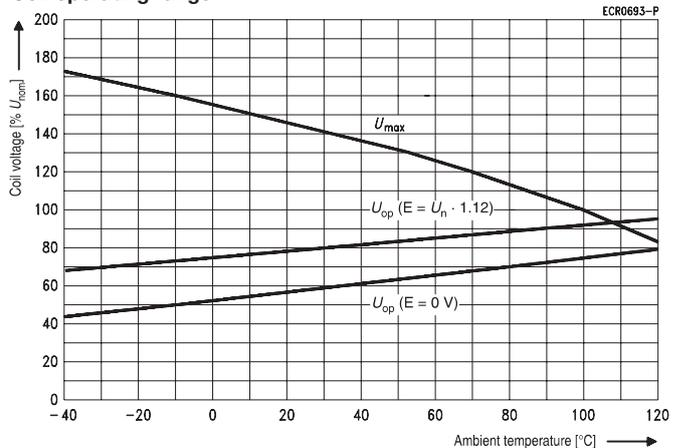
Does not take into account the temperature rise due to the contact current
