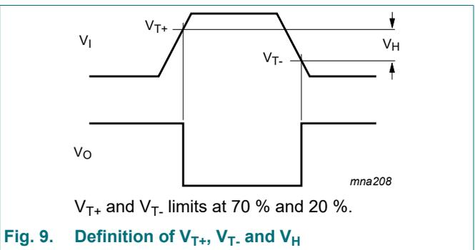
Fig. 9. Definition of V<sub>T+</sub>, V<sub>T-</sub> and V<sub>H</sub>
