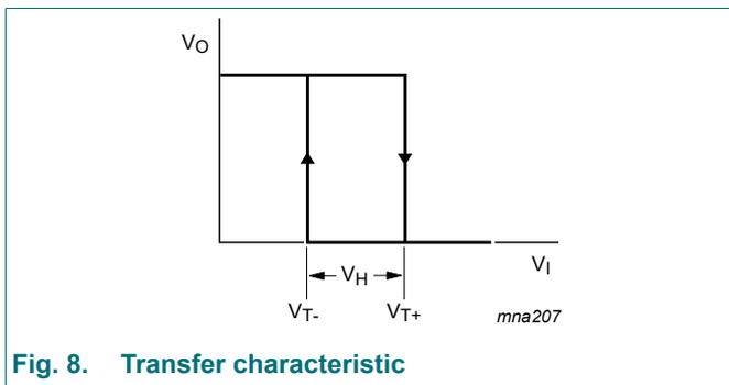
Fig. 8. Transfer characteristic
