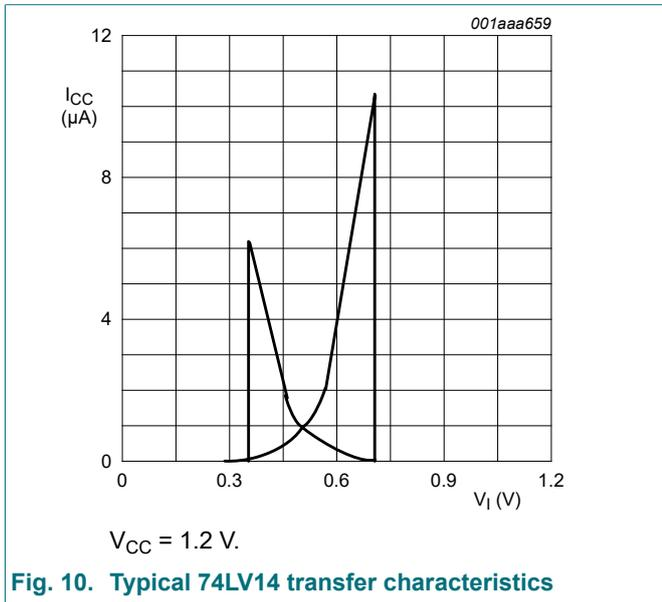
Fig. 10. Typical 74LV14 transfer characteristics
