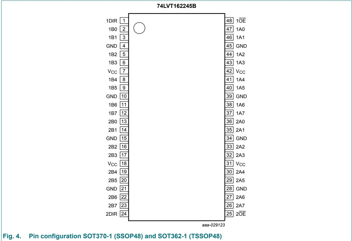
Fig. 4. Pin configuration SOT370-1 (SSOP48) and SOT362-1 (TSSOP48)
