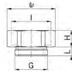
OUTER THREAD PG / INNER THREAD METRIC / WITH O-RING
