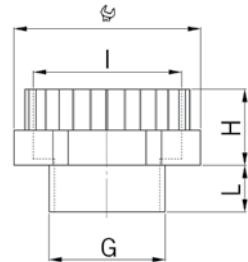
OUTER THREAD PG / INNER THREAD METRIC / LIGHT GREY RAL 7035
