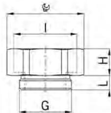
OUTER THREAD METRIC / INNER THREAD METRIC / WITH O-RING
