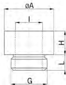
OUTER THREAD PG / INNER THREAD METRIC / WITHOUT O-RING
