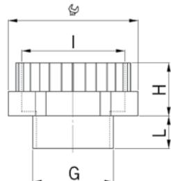
OUTER THREAD METRIC / INNER THREAD METRIC / LIGHT GREY RAL 7035
