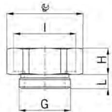
OUTER THREAD NPT / INNER THREAD PG / WITHOUT O-RING
