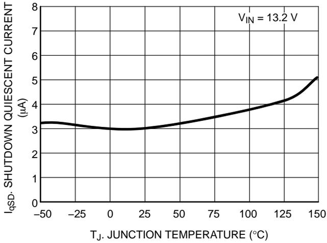
Figure 4. Shutdown Quiescent Current vs. Junction Temperature
