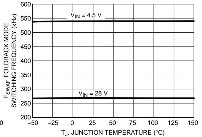
Figure 19. Short-Circuit Foldback Frequency vs. Junction Temperature
