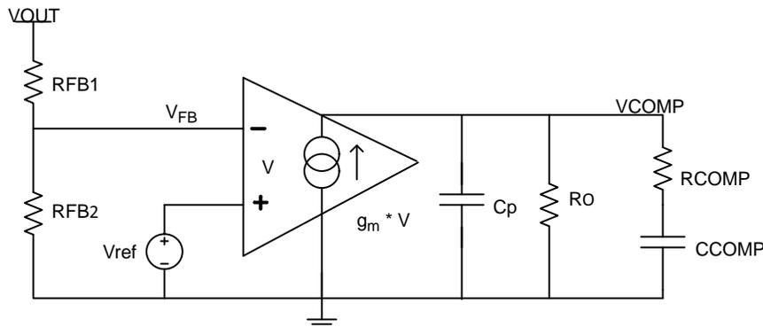
Figure 32. Feedback Compensator Network Model
