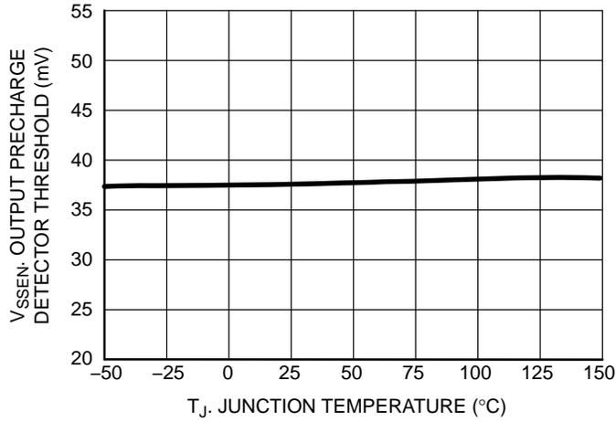
Figure 24. Output Precharge Detector Threshold vs. Junction Temperature
