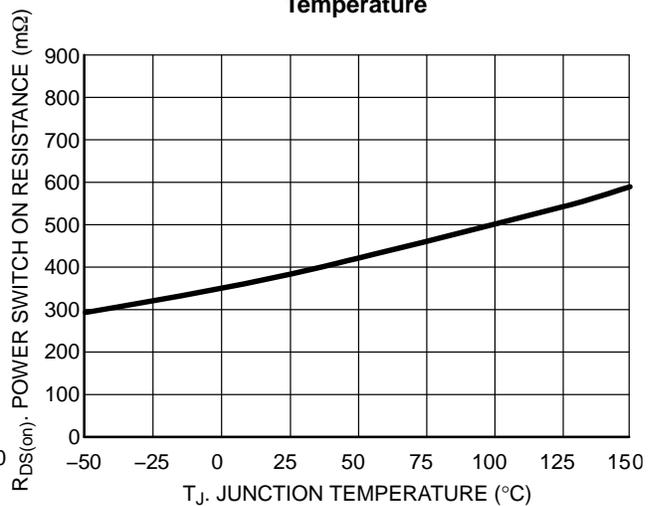
Figure 15. Power Switch  $R_{DS(on)}$  vs. Junction Temperature
