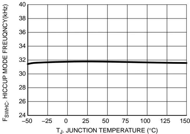
Figure 20. Hiccup Mode Frequency vs. Junction Temperature
