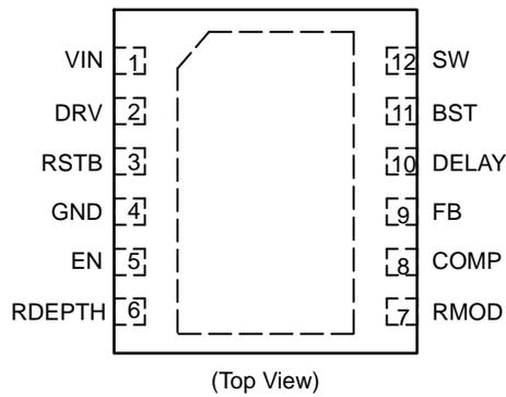
**Figure 3. Pin Connections**
