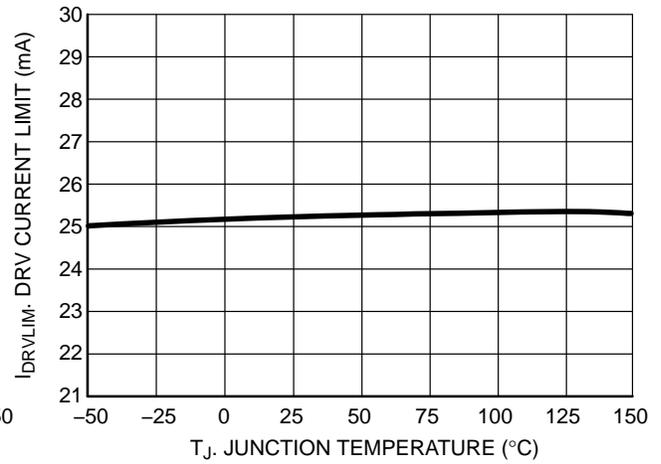
Figure 23. DRV Current Limit vs. Junction Temperature
