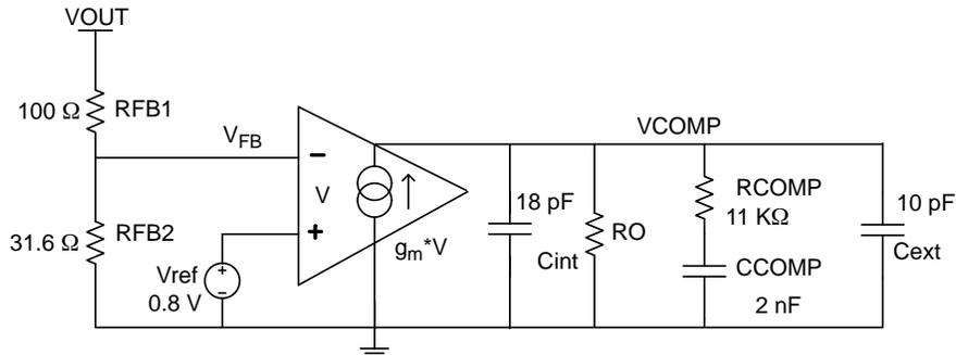
Figure 34. Example of the Feedback Compensation Network
