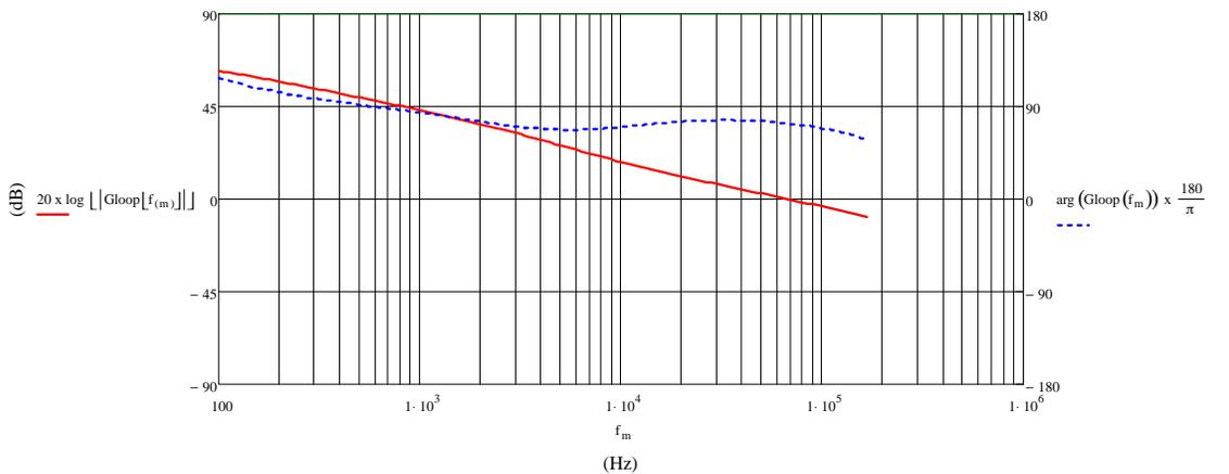
**Figure 36. Bode Plot of the Total Loop**
