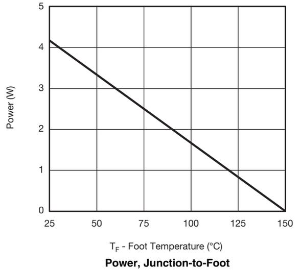
\* The power dissipation  $P_D$  is based on  $T_{J(max)} = 150$  °C, using junction-to-case thermal resistance, and is more useful in settling the upper dissipation limit for cases where additional heatsinking is used. It is used to determine the current rating, when this rating falls below the package limit.
