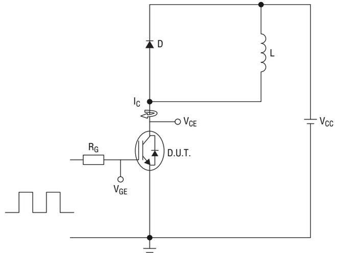
$L = 2.8 \text{ mH}$ ,  $V_{CE} = 400 \text{ V}$ ,  $V_{GE} = 15 \text{ V}$ ,  $I_C = 20 \text{ A}$ ,  $R_G = 10 \Omega$
