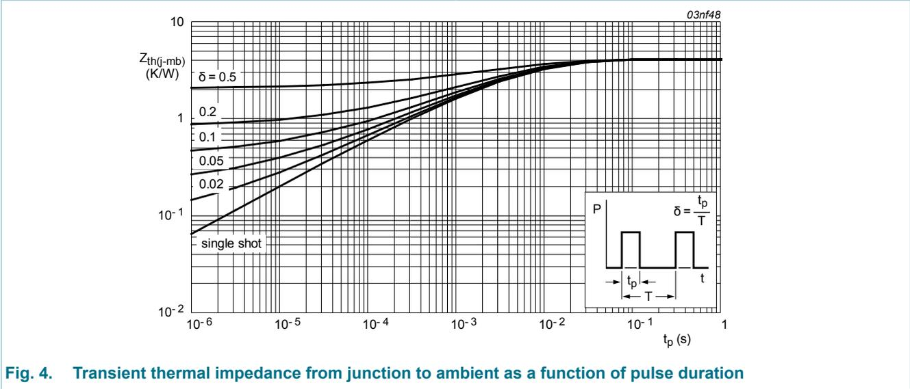
Fig. 4. Transient thermal impedance from junction to ambient as a function of pulse duration
