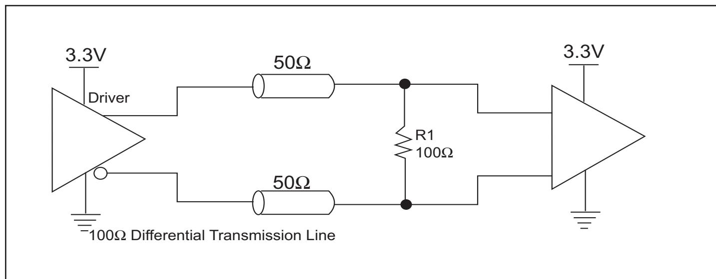
A general interface is shown above. In a 100Ω differential transmission line environment, drivers require a matched load termination of 100Ω across near the receiver input.
