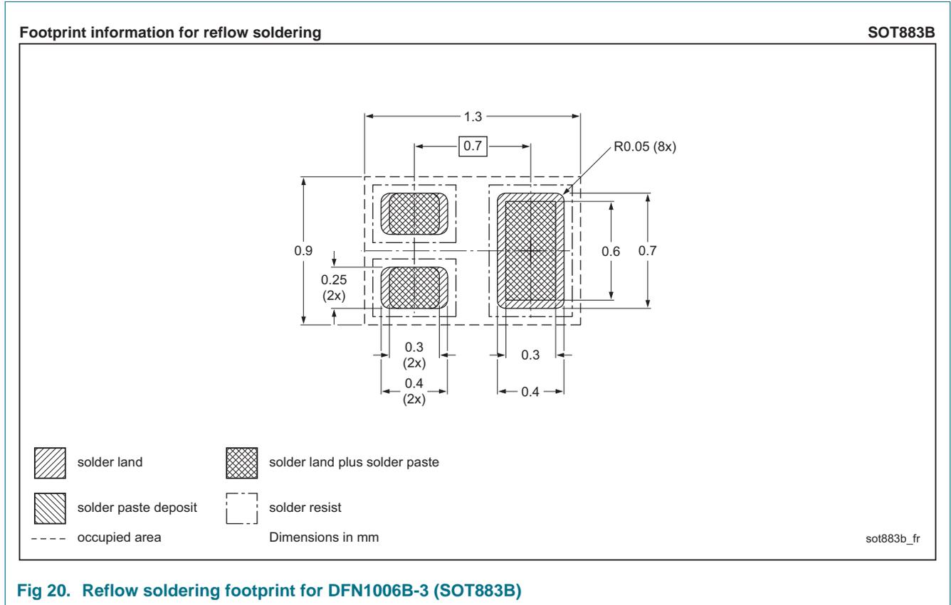
Fig 20. Reflow soldering footprint for DFN1006B-3 (SOT883B)
