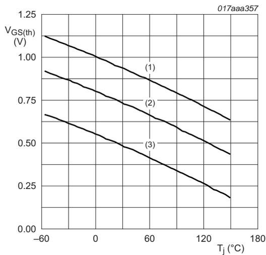
$I_D = 0.25\text{ mA}; V_{DS} = V_{GS}$
