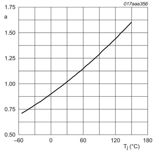
$$a = \frac{R_{DS(on)}}{R_{DS(on)(25^\circ C)}}$$
