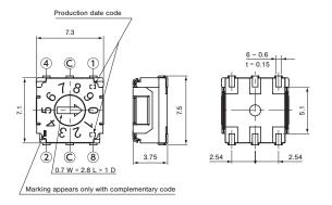
Unless otherwise specified, tolerance: ± 0.3 (Unit: mm)
