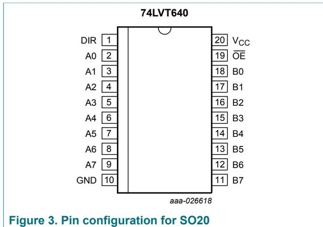
Figure 3. Pin configuration for SO20
