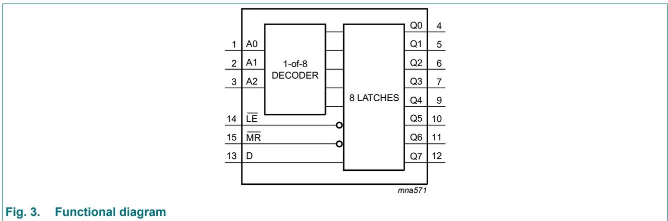
Fig. 3. Functional diagram
