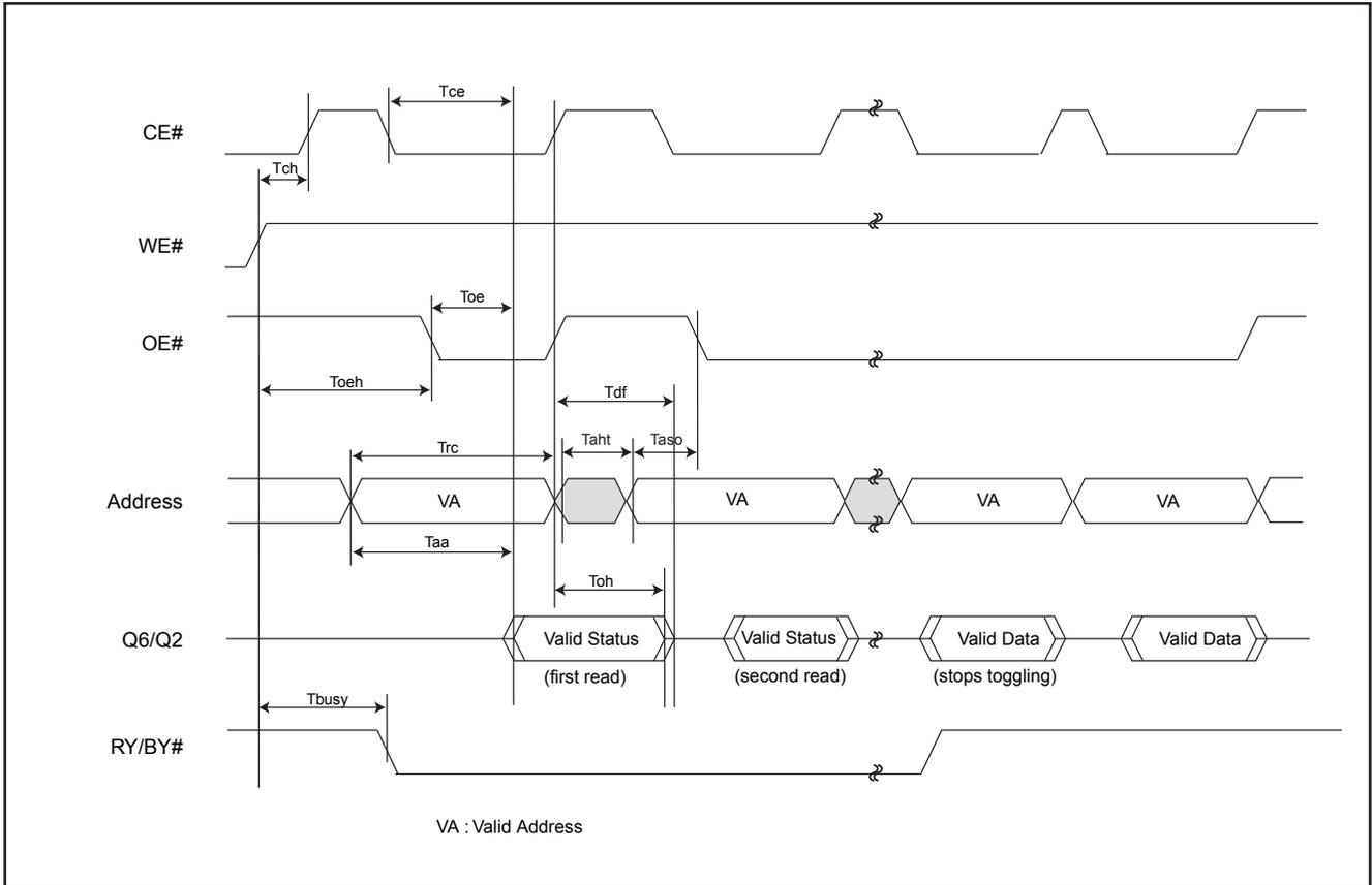
**Figure 21. TOGGLE BIT ALGORITHM**
