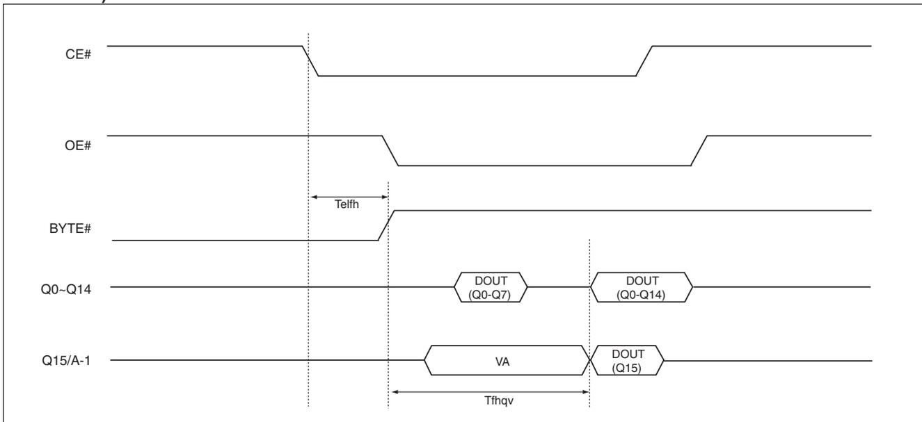
**Figure 23. PAGE READ TIMING WAVEFORM**
