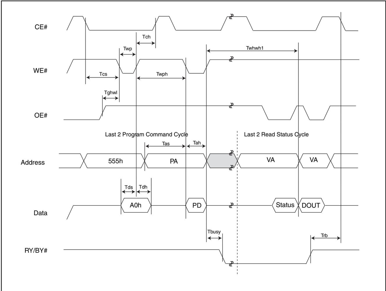
**Figure 13. ACCELERATED PROGRAM TIMING DIAGRAM**
