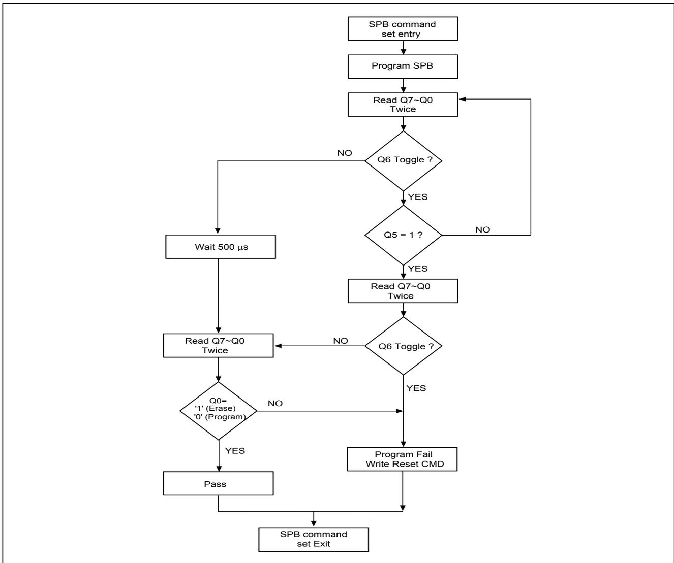
Note: SPB program/erase status polling flowchart: check Q6 toggle, when Q6 stop toggle, the read status is 00H /01H (00H for program/ 01H for erase), otherwise, the status is "fail" and "exit".
