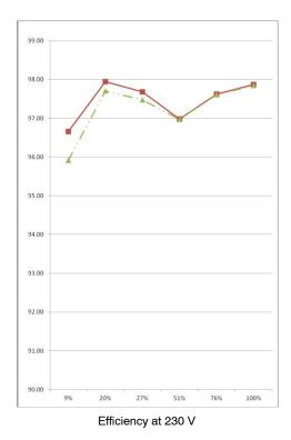
Figure 10. Efficiency versus Load of the Evaluation Board (red solid line) and of the Evaluation Board where Skip Mode is Disabled (green dotted line). In both Cases, the NTC is Shorted.
