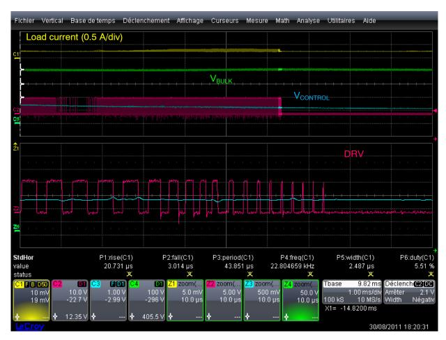
Figure 16. Soft Over-Voltage Protection
