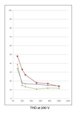
Figure 12. Total Harmonic Distortion (THD) versus Load of the Evaluation Board (red solid line), of the Evaluation Board where Skip Mode is Disabled (green dotted line) and of the Evaluation Board Operated in CrM.
