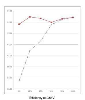
Figure 8. Efficiency versus Load of the Evaluation Board (red solid line), of the Evaluation Board Operated in Full CrM (purple dotted line). In both Cases, the NTC is Shorted.
