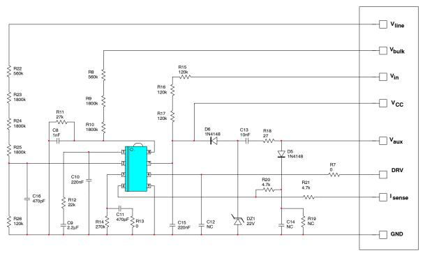
Figure 3. Application Schematic - Control Section
