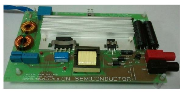
Figure 1. A Slim Board (Height < 13 mm)
