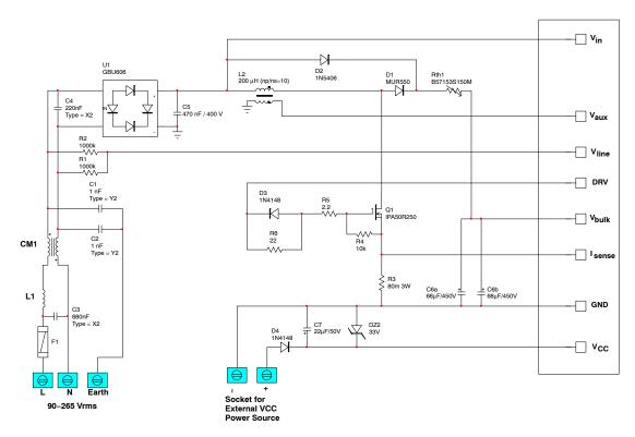
Figure 2. Application Schematic - Power Section
