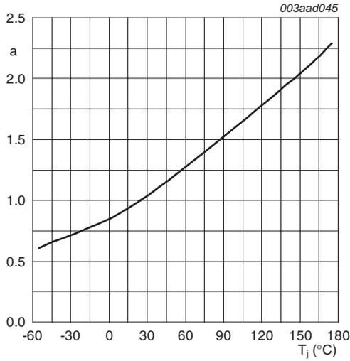
$$a = \frac{R_{DSon}}{R_{DSon(25^\circ C)}}$$
