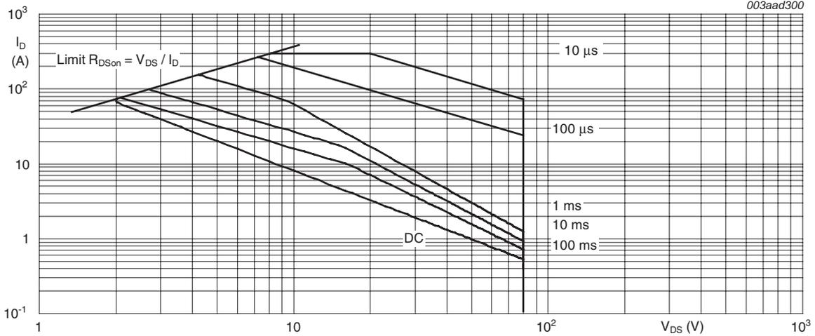
$T_{mb} = 25\text{ }^\circ\text{C}; I_{DM}$  is single pulse
