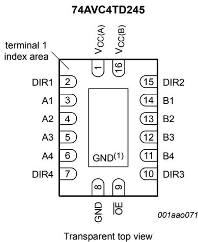
(1) This is not a supply pin, the substrate is attached to this pad using conductive die attach material. There is no electrical or mechanical requirement to solder this pad however if it is soldered the solder land should remain floating or be connected to GND.
