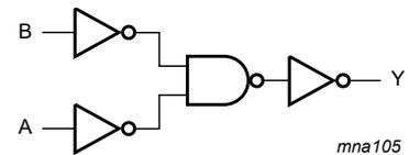
Fig. 3. Logic diagram
