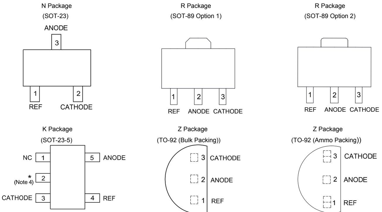
Note: 4. \* Pin 2 is attached to substrate and must be connected to ANODE or open.
