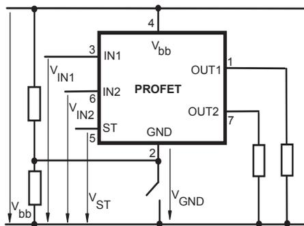
Any kind of load. If  $V_{GND} > V_{IN} - V_{IN(T+)}$  device stays off
