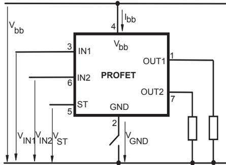
Any kind of load. In case of Input=high is  $V_{OUT} \approx V_{IN} - V_{IN(T+)}$ .
