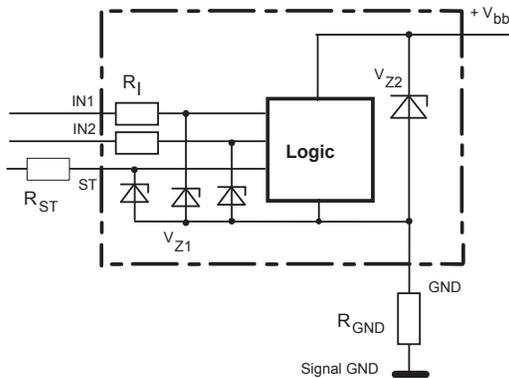
$V_{Z1} = 6.1$  V typ.,  $V_{Z2} = 47$  V typ.,  $R_1 = 3.5$  k $\Omega$  typ.,  $R_{GND} = 150$   $\Omega$
