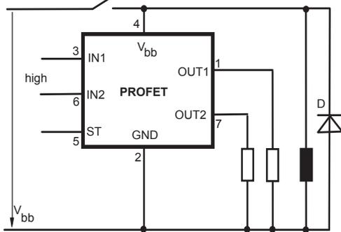
If other external inductive loads L are connected to the PROFET, additional elements like D are necessary.
