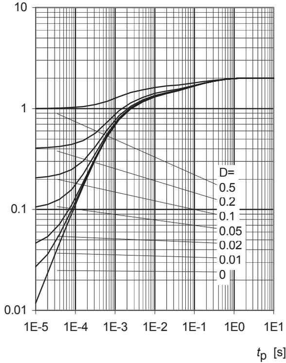
**Transient thermal impedance chip case**
