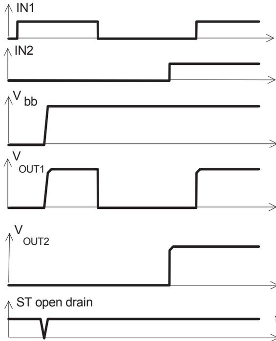
**Figure 2b:** Switching an inductive load
