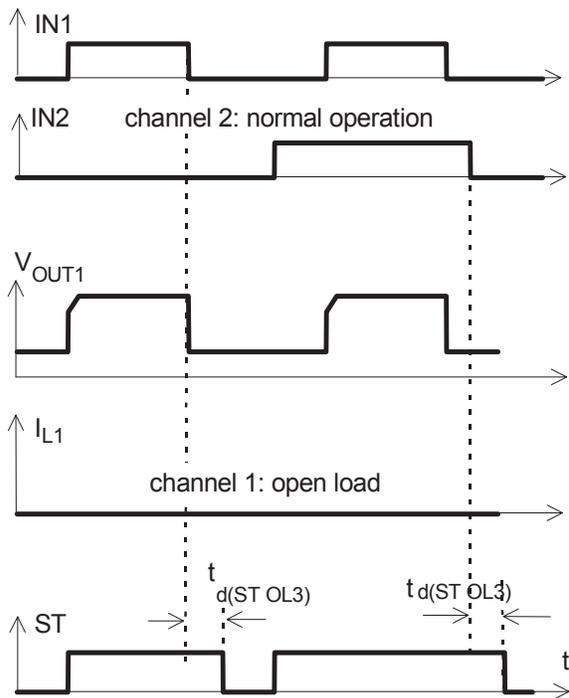
$t_{d(ST,OL3)}$  depends on external circuitry because of high impedance
