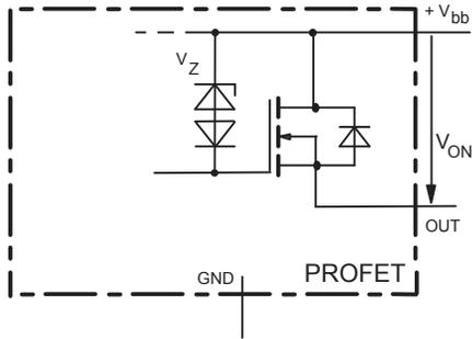
$V_{ON}$  clamped to 47 V typ.
