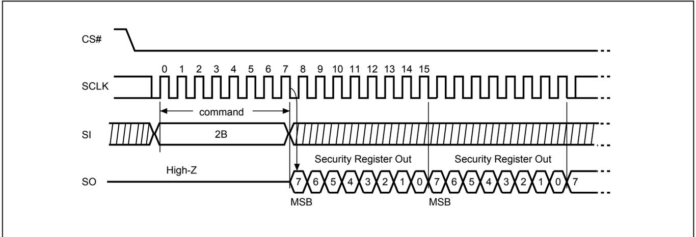
**Figure 28. Write Security Register (WRSCUR) Sequence (Command 2F)**
