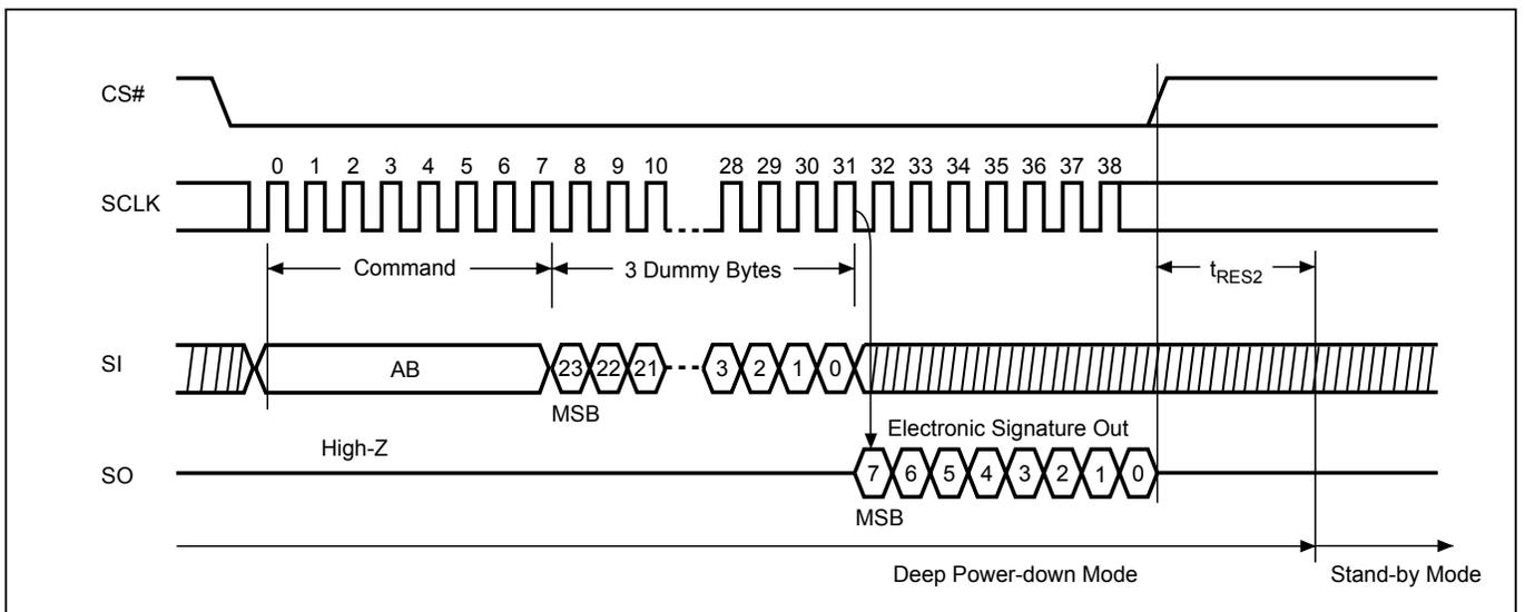
**Figure 25. Read Identification (RDID) Sequence (Command 9F)**
