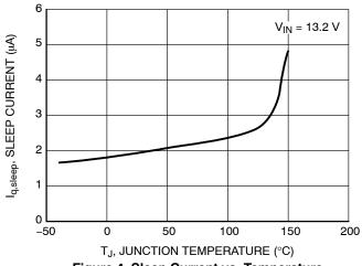
Figure 4. Sleep Current vs. Temperature
