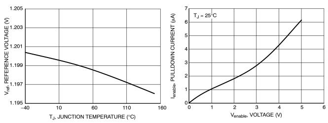
Figure 8. Reference Voltage vs. Temperature
