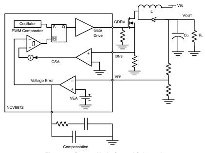
Figure 11. Current Mode Control Schematic
