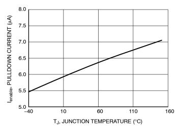
Figure 10. Enable Pulldown Current vs. Temperature
