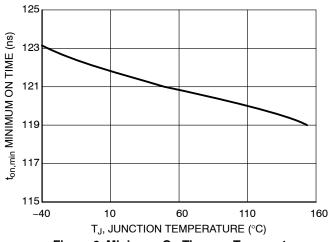
Figure 6. Minimum On Time vs. Temperature
