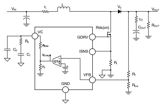
Figure 12. NCV887200 Boost Converter OTA and Compensation
