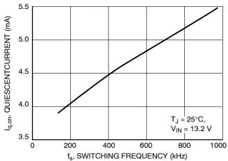
Figure 3. Quiescent Current vs. Switching Frequency
