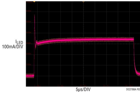
$V_{IN} = 12V$ ,  $V_{LED} = 24V$ ,  $I_{LED} = 330mA$
