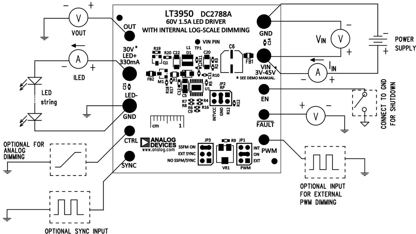
Figure 1. Test Procedure Setup Drawing for DC2788A
