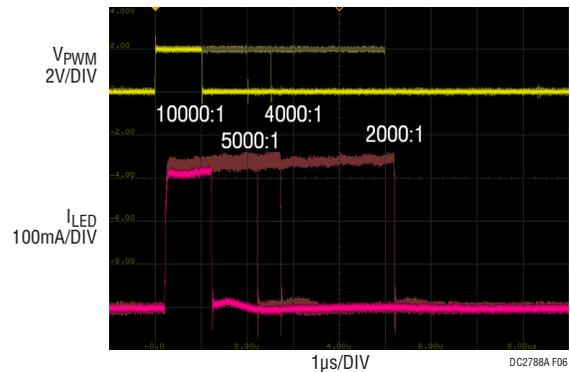
$V_{IN} = 12V$ ,  $V_{LED} = 24V$ ,  $I_{LED} = 330mA$
