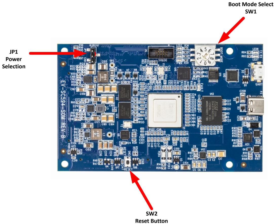
Figure 3-6: Switch/Jumper Locations
