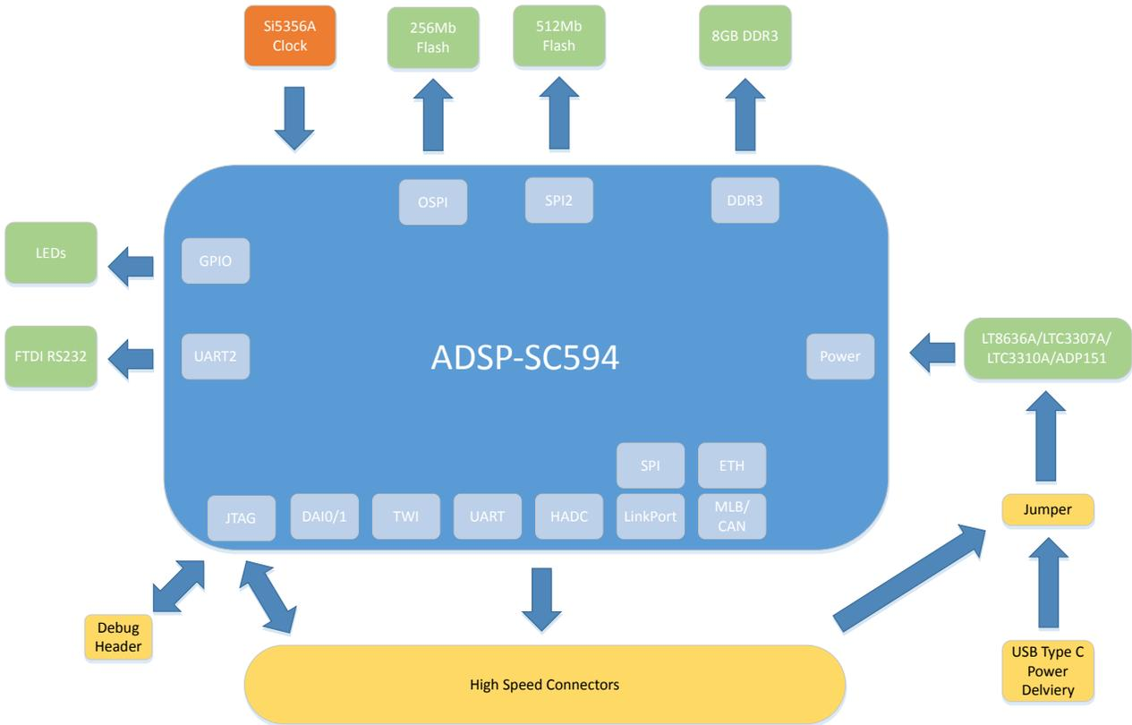
Figure 3-1: Block Diagram
