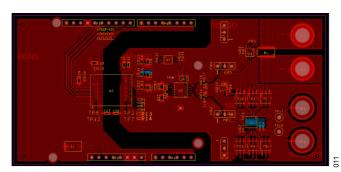
Figure 10. Top layer PCB isolation
