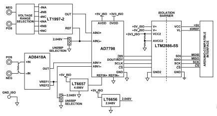
Figure 1. CN0548 Block Diagram
