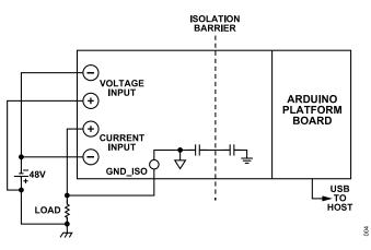
Figure 4. -48 V Voltage and current measurement
