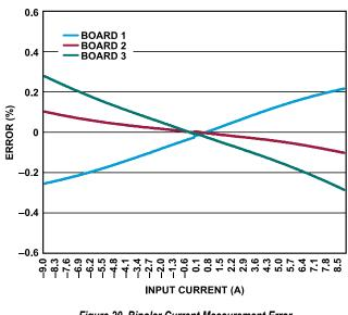
Figure 20. Bipolar Current Measurement Error
