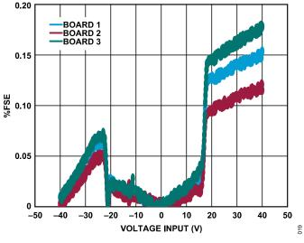
Figure 16. Bipolar Accuracy (Uncalibrated)
