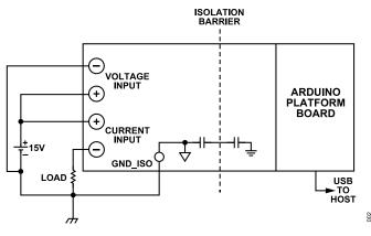
Figure 2. +15 V High side Current and Voltage Measurement
