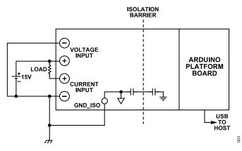
Figure 3. +15 V Low side Current and Voltage Measurement
