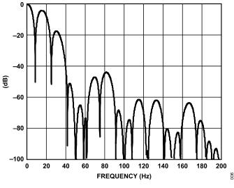
Figure 8. AD7798 Filter Response, 16.7 Hz Update Rate Mode
