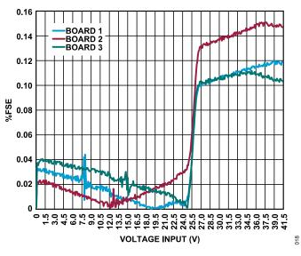
Figure 15. Unipolar Accuracy (Uncalibrated)
