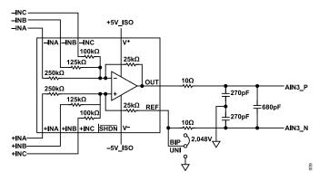
Figure 6. Voltage Range and Polarity Circuitry
