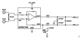
Figure 7. Current Input Signal Conditioning and Polarity Circuitry
