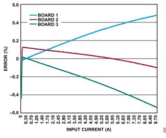
Figure 19. Unipolar Current Measurement Error
