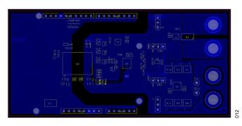
Figure 11. Bottom layer PCB isolation
