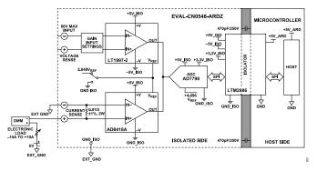
Figure 17. Current Input Test Setup
