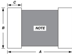
Note: Avoid metal runs in this area, parts are not recommended for use in applications using Silver (Ag) epoxy paste.
