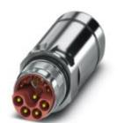
Coupling connector, straight long, shielded: yes, for standard and SPEEDCON interlock, M23, No. of pos.: 8+4+PE, type of contact: Pin, Crimp connection, cable diameter range: 12 mm ... 15 mm
