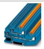
Feed-through terminal block, Connection method: Quick connection, Spring-cage connection, Cross section: 0.25 mm² - 1.5 mm², Width: 5.2 mm, Color: blue, Mounting: NS 35/7,5, NS 35/15 / Ex data new / /
