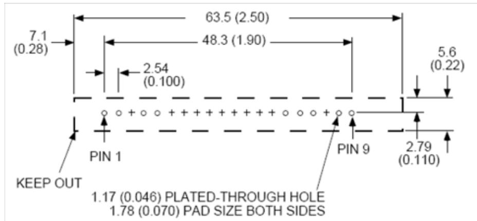
Note: No copper should be placed between pins 2 and 3 and pins 7 and 8.
