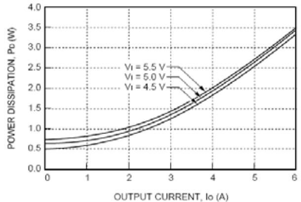
**Figure 30. NH020Y Power Dissipation vs. Output Current.**
