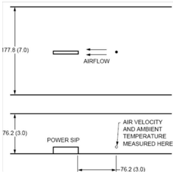
Note: Dimensions are in millimeters and (inches).
