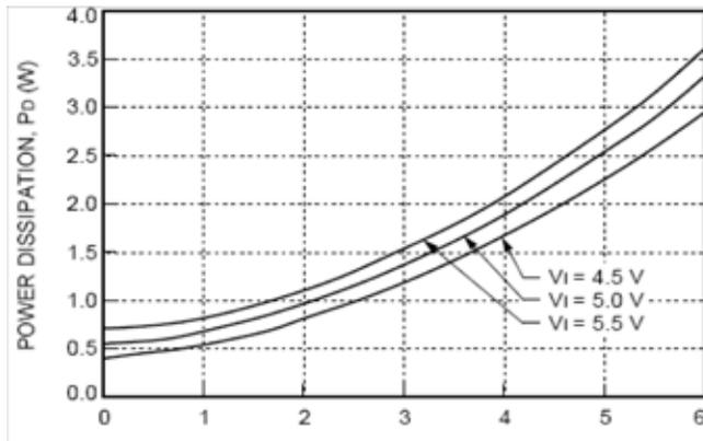
Figure 32. NH020F Power Dissipation vs. Output Current.
