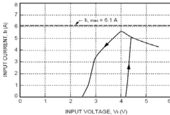
Figure 1. Typical Input Characteristics at 6 A output current.
