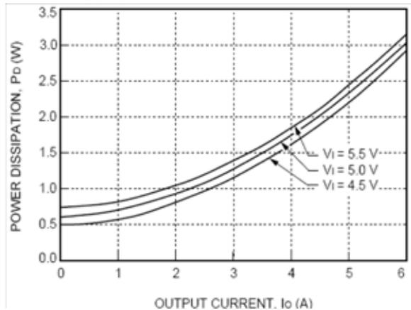
**Figure 31. NH020G Power Dissipation vs. Output Current.**
