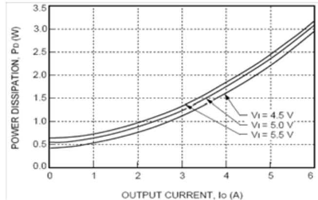
**Figure 29. NH020M Power Dissipation vs. Output current.**
