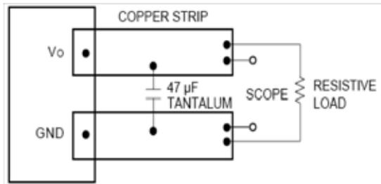
Note: Scope measurements should be made using a BNC socket, with a 47 µF tantalum capacitor. Position the load between 51 mm and 76 mm (2 in and 3 in) from the module
