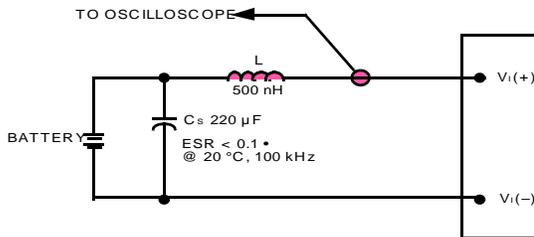
Note: Measure input reflected ripple current with a simulated source inductance ( $L_{TEST}$ ) of 500nH. Capacitor  $C_S$  offsets possible battery impedance. Measure current as shown above.
