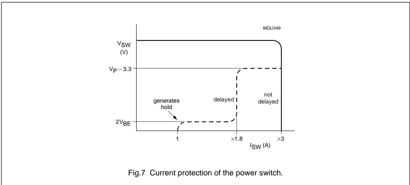
Fig.7 Current protection of the power switch.
