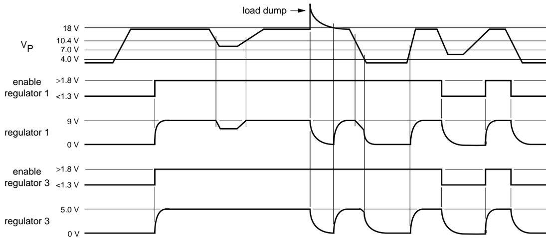
V<sub>P</sub> and enable Schmitt trigger
