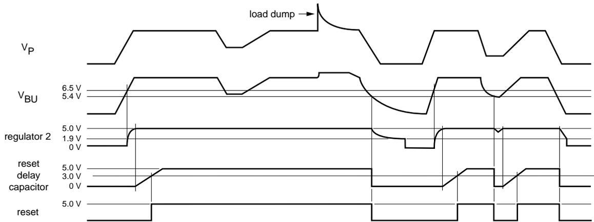
Backup Schmitt trigger and reset behaviour
