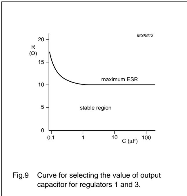
Fig.9 Curve for selecting the value of output capacitor for regulators 1 and 3.
