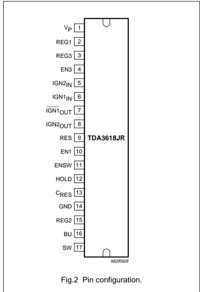
Fig.2 Pin configuration.
