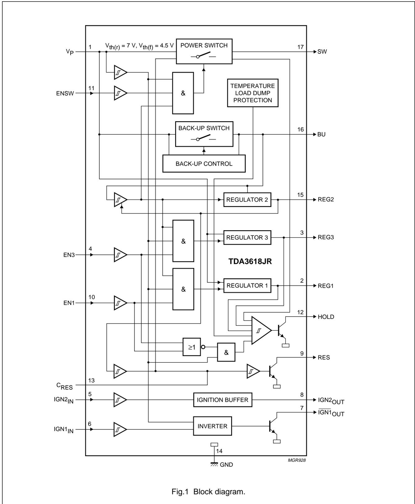
Fig.1 Block diagram.
