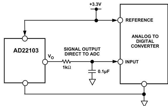
Figure 1. Application Circuit
