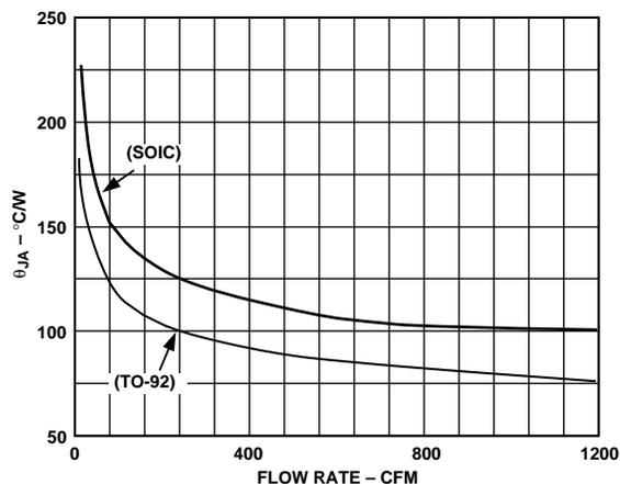
Figure 3. Thermal Resistance vs. Air Flow Rate
