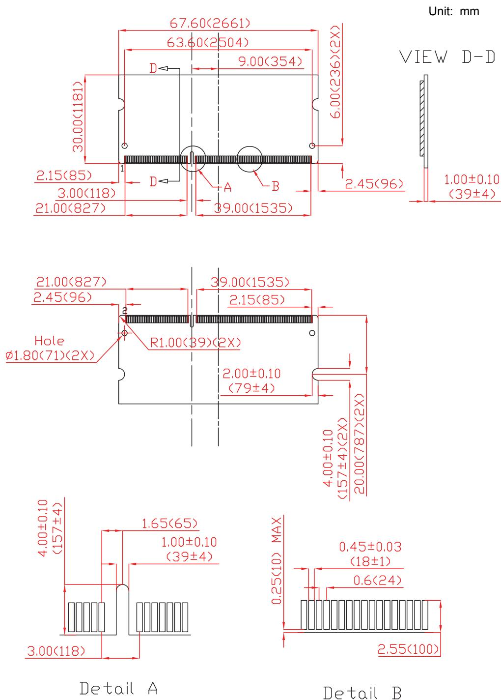
(All dimensions are in millimeters with ±0.15mm tolerance unless specified otherwise.)
