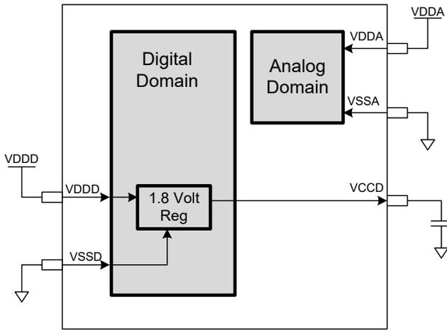
The PSoC 4100 family allows two distinct modes of power supply operation: Unregulated External Supply, and Regulated External Supply modes.
