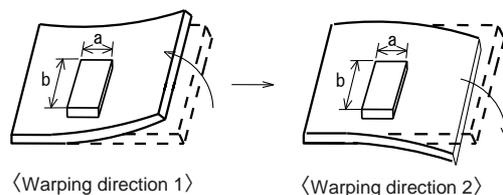
roducts(warping direction 1, warping direction 2) shall be located carefully so that products are not subject to the mechanical stress due to warping the board. Because they may be subjected the mechanical stress in order of warping direction 1>warping direction 2.
