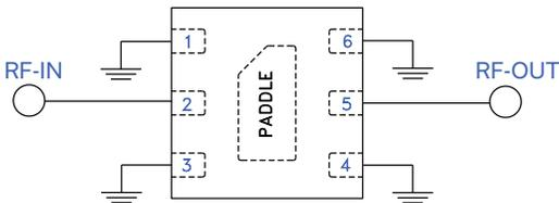
Fig 1. Block Diagram of Test Circuit used for characterization. Test Board TB-EQY-9-453+
