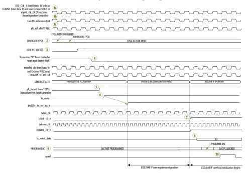
The recommended FPGA - DAC subsystem bring-up sequence:
