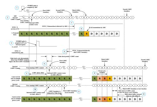
You should set a safe LMFC offset value to ensure deterministic latency from one power cycle to another power cycle. In Figure 30 on page 154, the illegal <code>csr\_Imfc\_offset</code> values of 1, 2, and 3 causes lane de-skew error because the RBD buffer size has exceeded.
