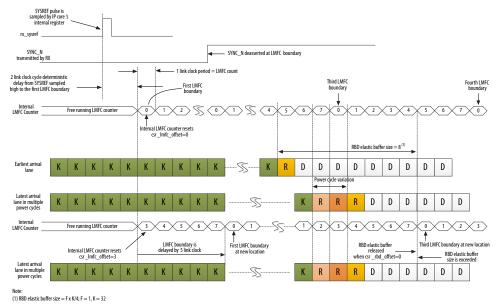
You can use the TX LMFC offset to align the LMFC counter in IP core to the LMFC counter in DAC.
