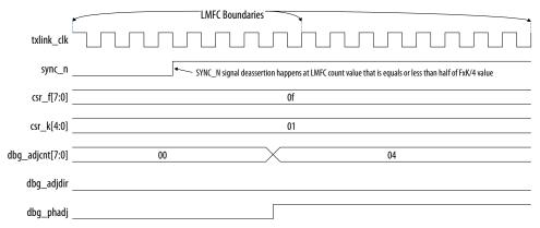
Figure 16. Timing Diagram Example for Case 3
