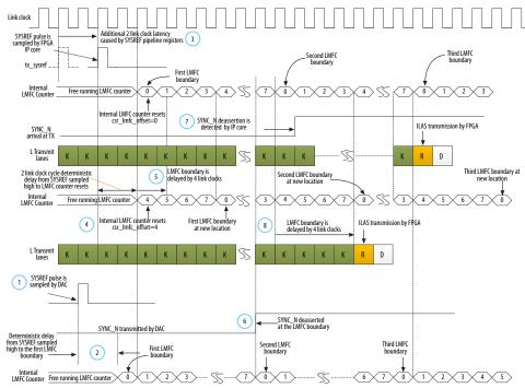
The *csr\_lmfc\_offset* field provides a convenient way to achieve deterministic latency and potentially optimizing the IP core latency. There are other ways that you can achieve deterministic latency by using the features available at the converters. Consult the converter manufacturer for details of these features.
