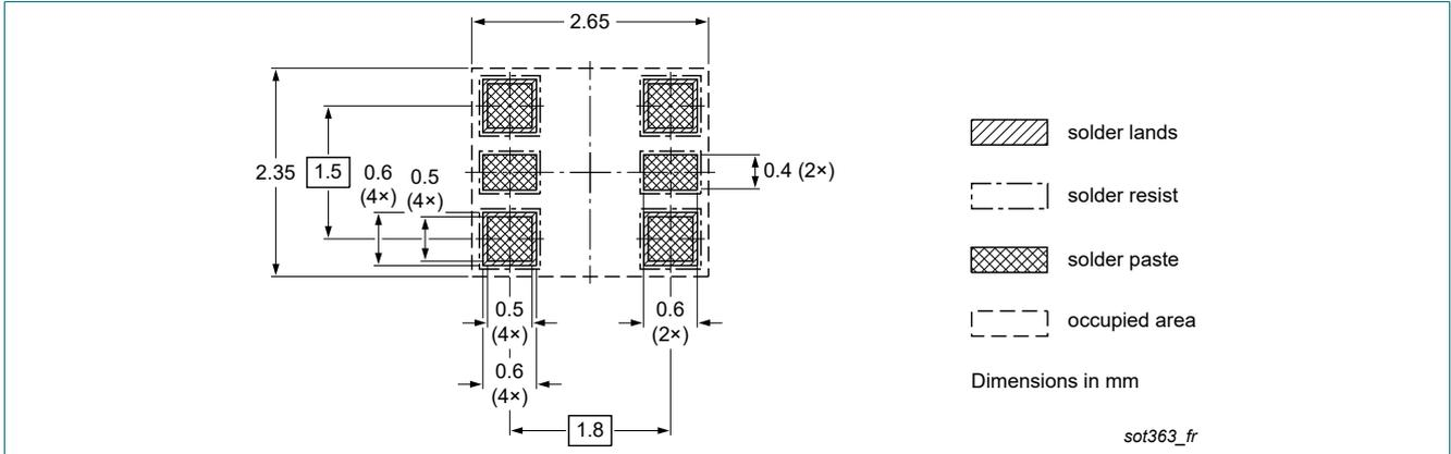
Fig. 14. Reflow soldering footprint for TSSOP6 (SOT363)
