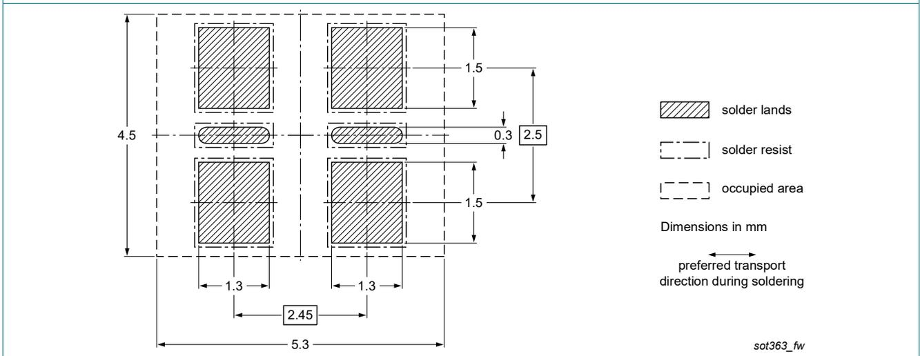
Fig. 15. Wave soldering footprint for TSSOP6 (SOT363)
