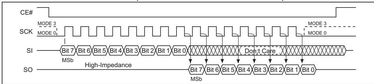
**FIGURE 4-2: SQI SERIAL QUAD I/O PROTOCOL**
