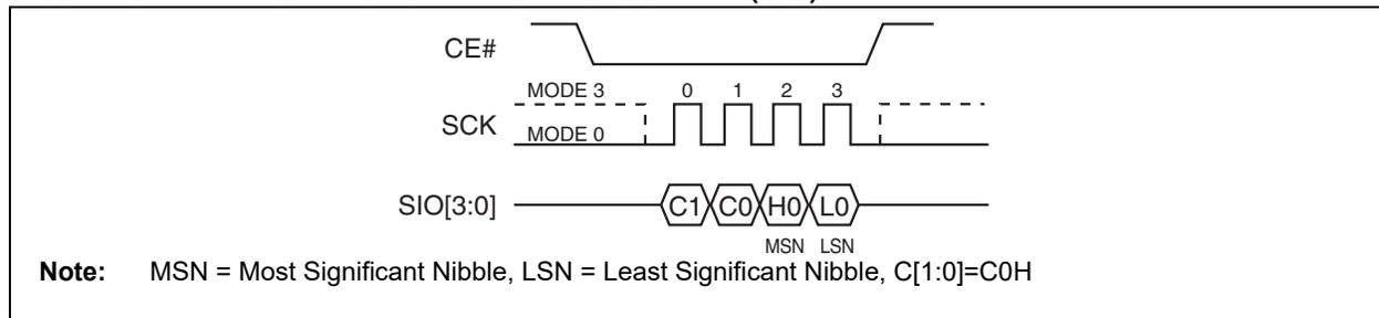
**FIGURE 5-12: SET BURST LENGTH SEQUENCE (SPI)**
