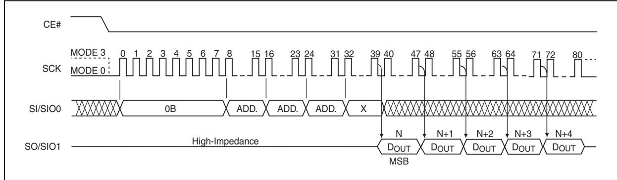
In SQI protocol, the host drives CE# low then send the Read command cycle command, 0BH, followed by three address cycles, a Set Mode Configuration cycle, and two dummy cycles. Each cycle is two nibbles (clocks) long, most significant nibble first.
