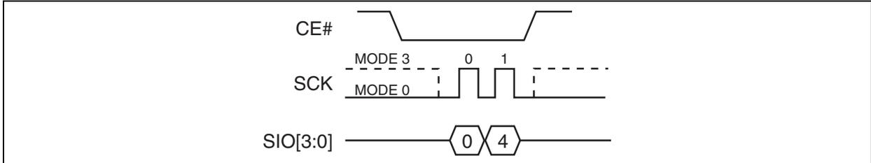
**FIGURE 5-35: WRITE DISABLE (WRDI) SEQUENCE (SPI)**
