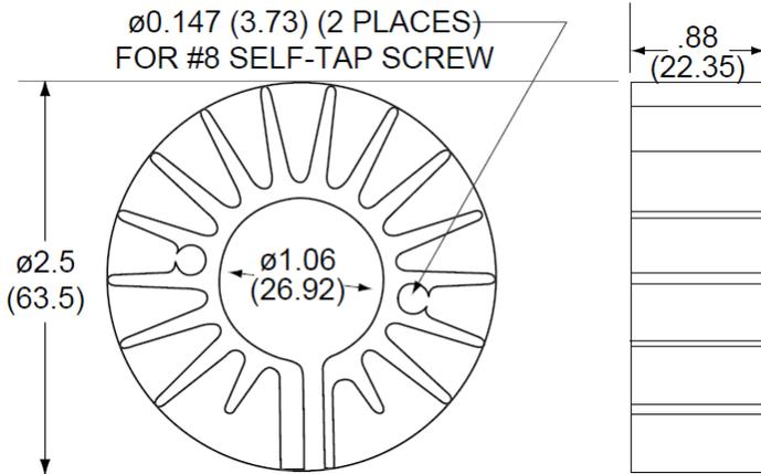
LS-1130 Optical Adapter (p/n: MVS-14-1) – Included with unit
