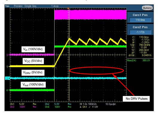
Figure 31. Startup with Jumper Removed (V<sub>in</sub> = 265 Vac 50 Hz, I<sub>out</sub> = 0 mA)
