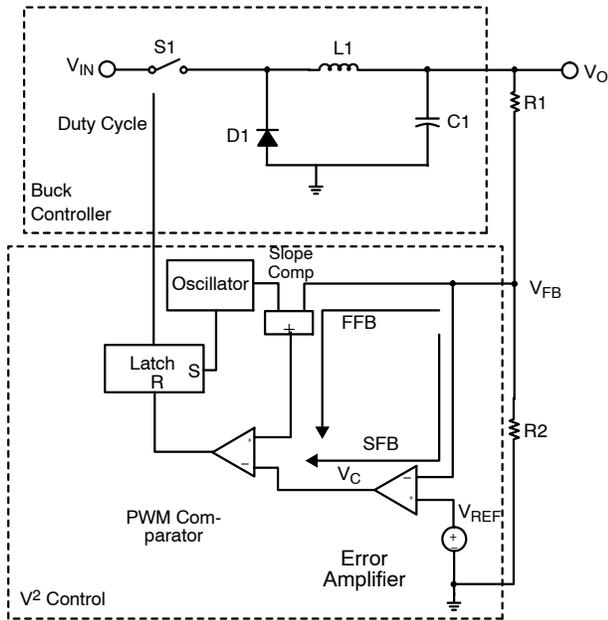
Figure 3. Buck Converter with V<sup>2</sup> Control.
