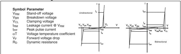
Figure 2. Pulse definition for electrical characteristics
