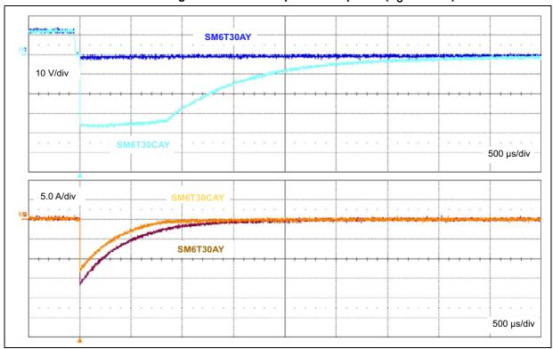
Figure 7. ISO 7637-2 pulse 2a response ( $V_S = 112 \text{ V}$ )
