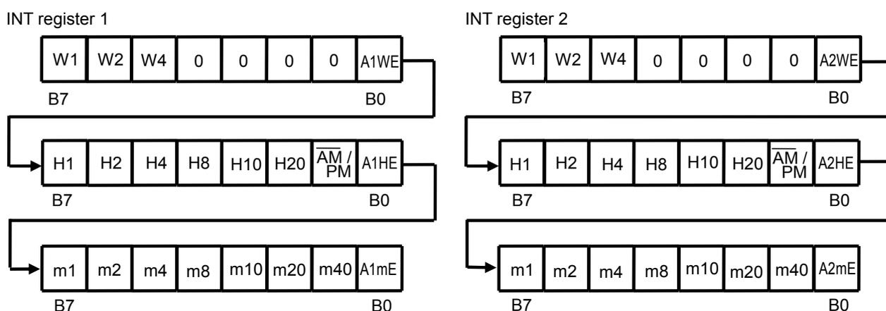
Figure 17 INT Register 1 and INT Register 2 (Alarm-Time Data)
