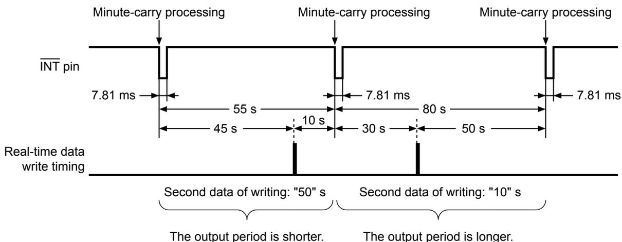
**Figure 32 Timing of Minute-periodical Interrupt Output 2**
