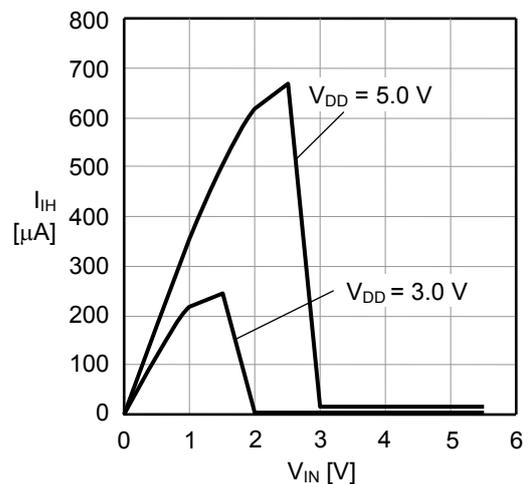
13. BLD detection, release voltage,  $V_{DDT}$  (min.)
