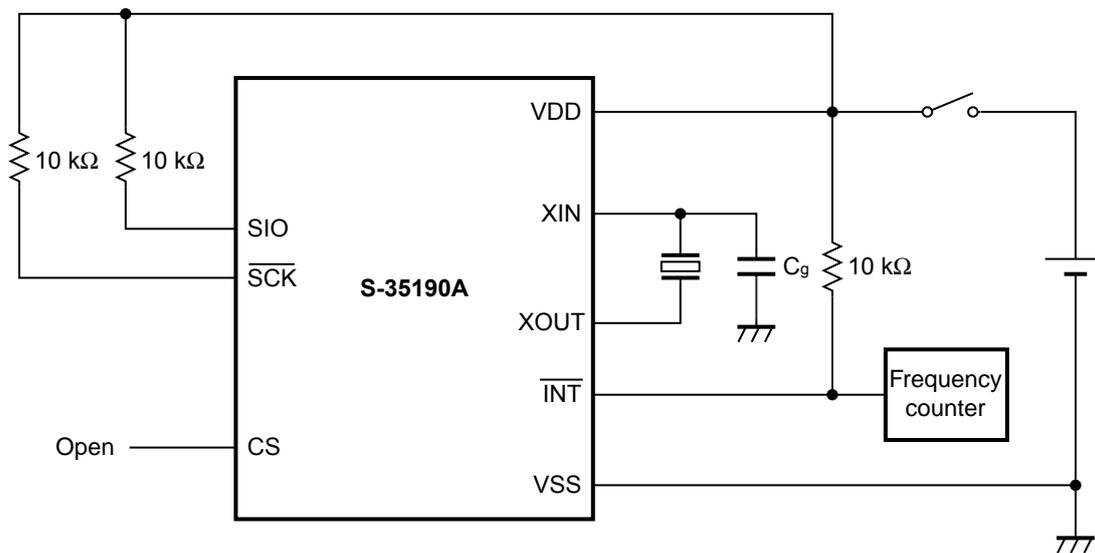
Figure 47 Configuration of Oscillation Frequency Measurement Circuit
