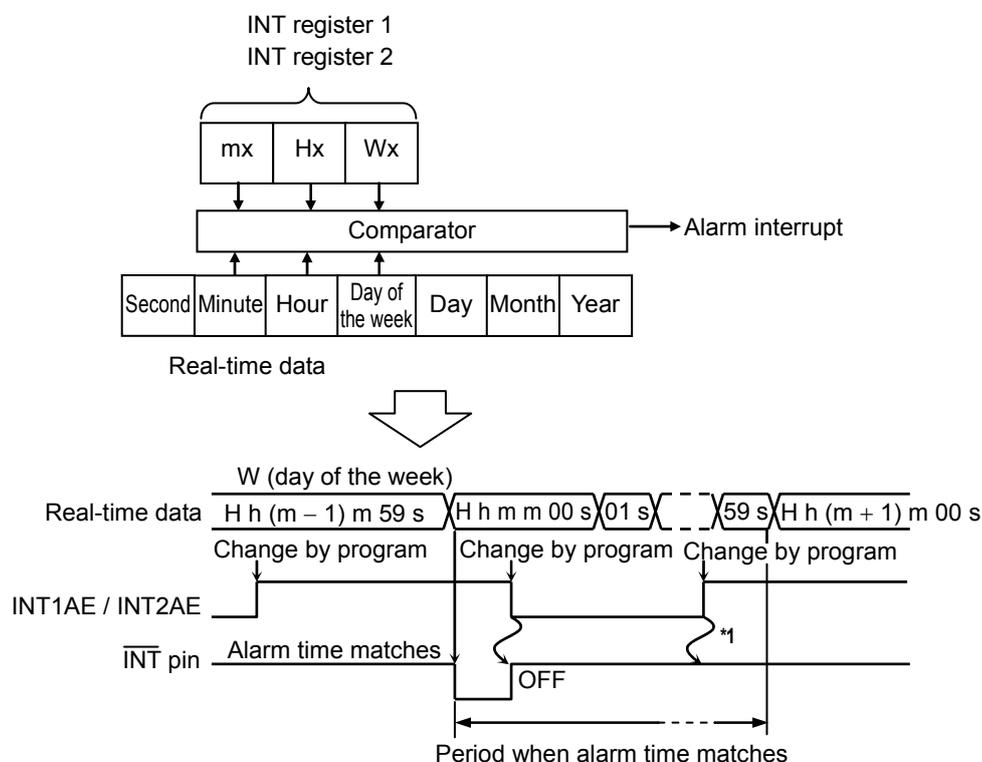
\*1. If users clear INT1AE / INT2AE once; "L" is not output from the  $\overline{\text{INT}}$  pin by setting INT1AE / INT2AE enable again, within a period when the alarm time matches real-time data.
