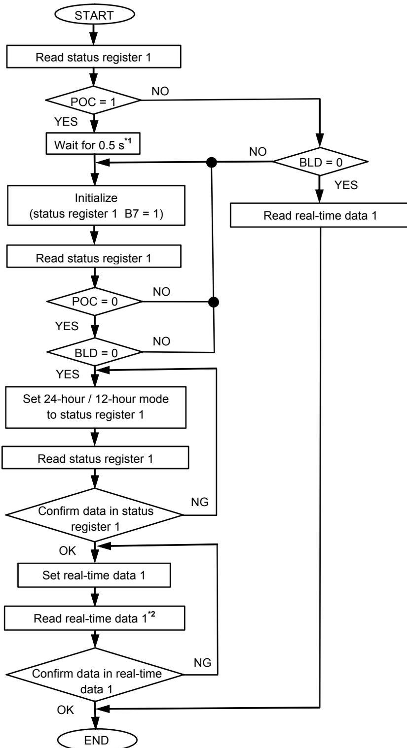
\*1. Do not communicate for 0.5 seconds since the power-on detection circuit is in operation.
