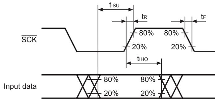
**Figure 11 Timing Diagram 2 during 3-wire Communication**
