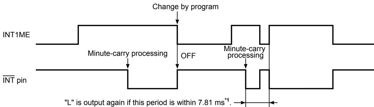
\*1. Pin output is set to "H" by disabling the output mode within 7.81 ms, because the signal of this procedure is maintained for 7.81 ms. Note that pin output is set to "L" by setting the output mode enable again.
