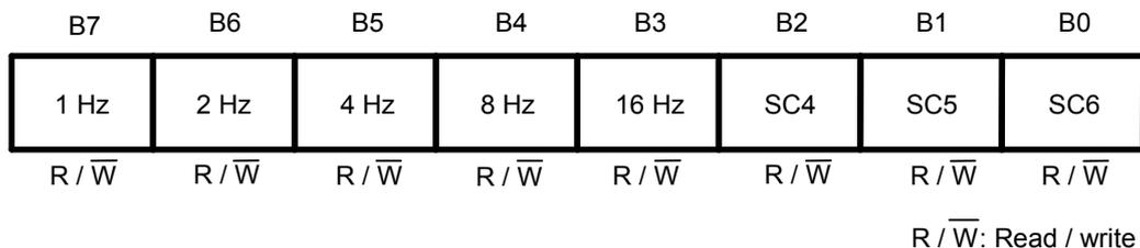
**Figure 18 INT Register 1 (Data Register for Output Frequency)**
