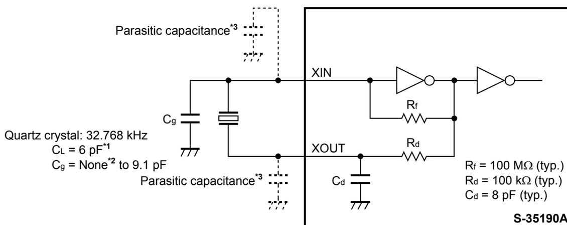
\*1. When setting the value for the quartz crystal's  $C_L$  as 7 pF, connect  $C_d$  externally if necessary.
