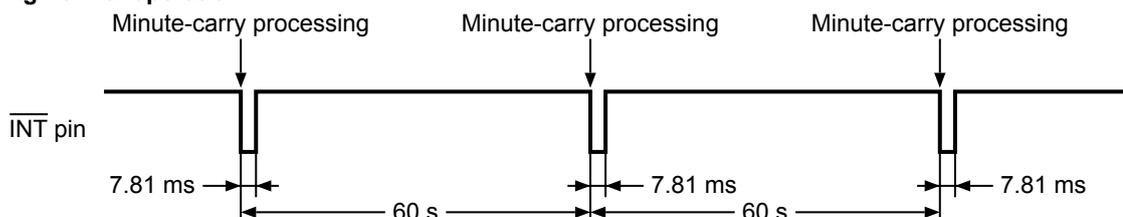
**(2) During reading operation in the real-time data register**
