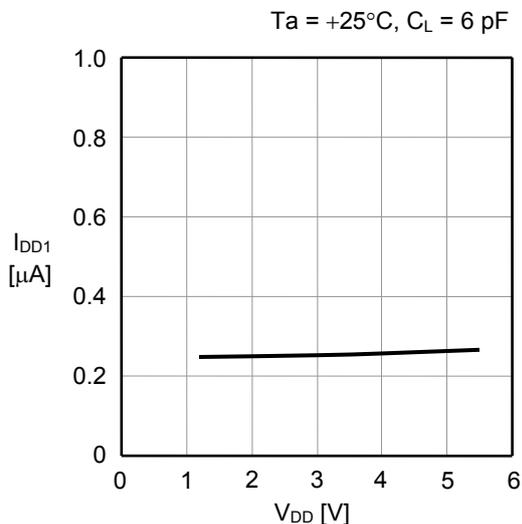
2. Current consumption when 32.768 kHz output vs.  $V_{DD}$  characteristics
