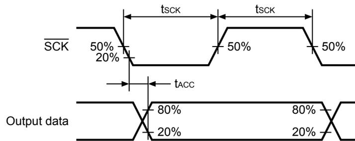
**Figure 12 Timing Diagram 3 during 3-wire Communication**
