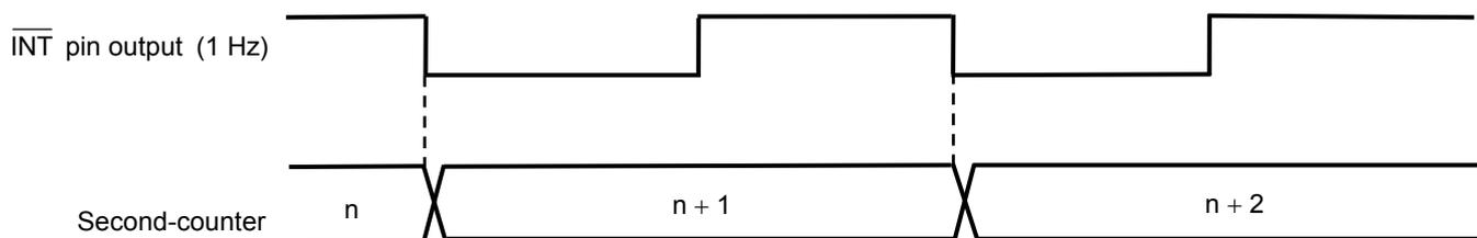
**Figure 20 1 Hz Clock Output and Second-counter**
