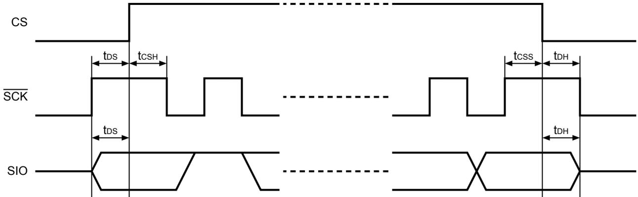
**Figure 10 Timing Diagram 1 during 3-wire Communication**
