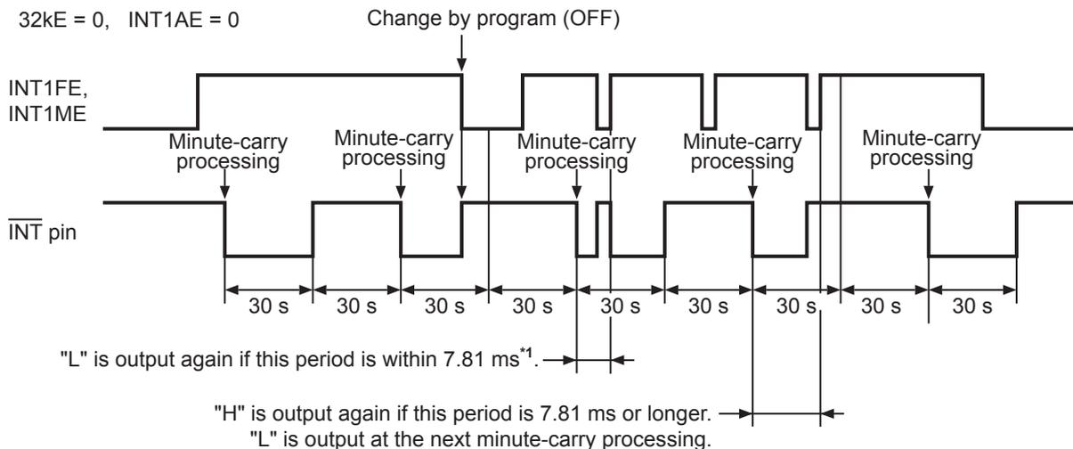
\*1. Setting the output mode disable makes the pin output "H", while the output from the  $\overline{\text{INT}}$  pin is in "L". Note that pin output is set to "L" by setting the output mode enable again.
