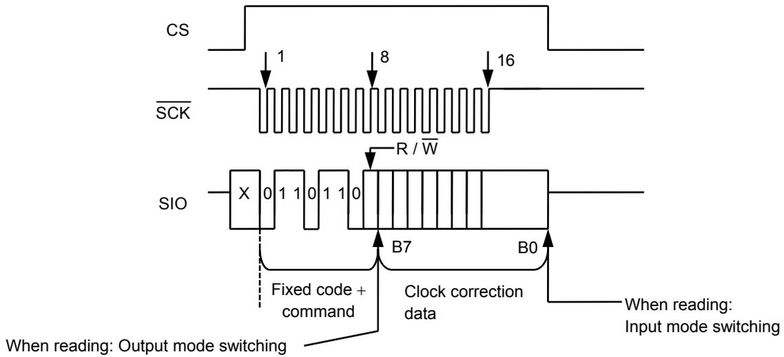
Figure 40 Clock Correction Register Access
