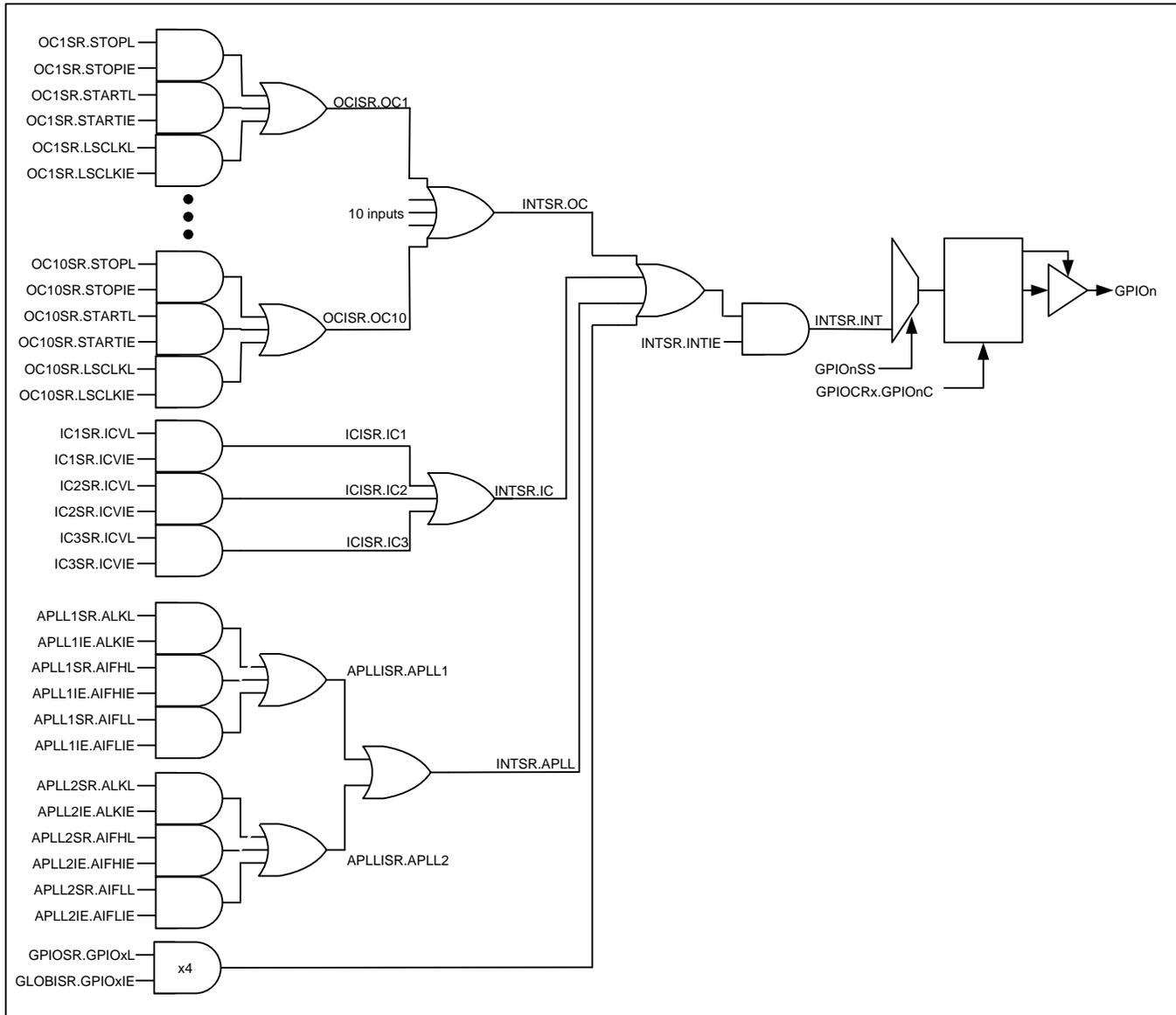
Figure 13 - Interrupt Structure
