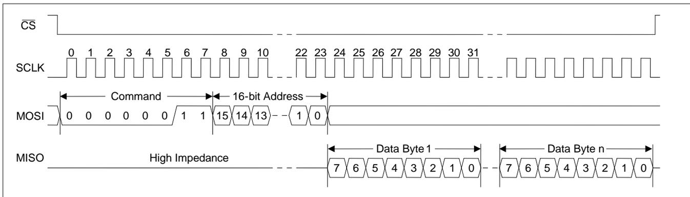
Figure 6 - SPI Read Transaction Functional Timing
