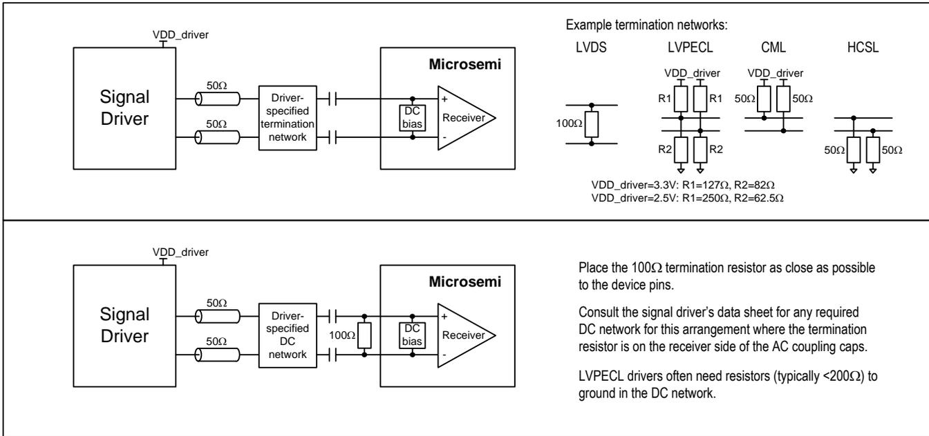
Figure 15 - Example External Components for Differential Input Signals
