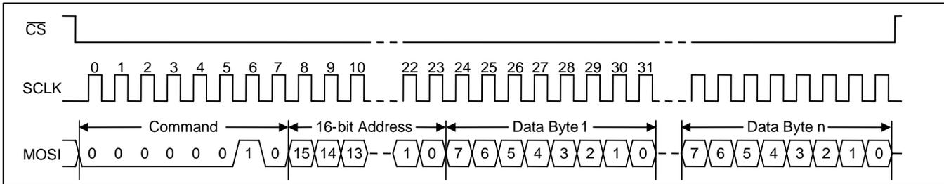
Figure 8 - SPI Write Transaction Functional Timing
