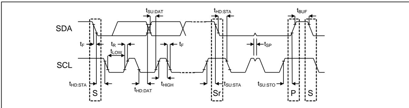
**Figure 20 - I<sup>2</sup>C Slave Interface Timing**
