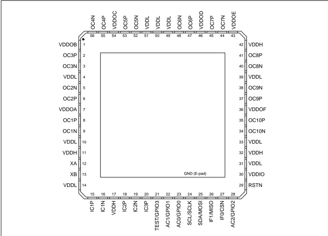
Figure 3 - Pin Diagram
