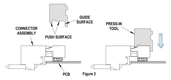
3. Using the application tool and an appropriate press, seat the Orthogonal Direct Ram module until there is less than 0.10mm (.004 in) clearance between the bottom of the plastic housing and the surface of the PCB. See Figure 3.
