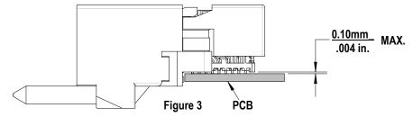
There should be no broken stand-offs along the perimeter of the part (an indication of over-pressing).
