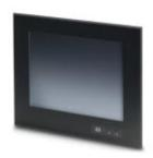
Touch panel with 30.7 cm/12.1" TFT-Display (Analog resistive (polyester)), 800 x 600 Pixel (SVGA), 65536 colors, Xscale® PXA320, 806 MHz, 2x USB host 1.1, 1x CompactFlash®, 1 x Ethernet (10/100 Mbps), RJ45, Windows CE 6.0 and User software: Visu+ / AX OPC Server. (Bus system: without)
