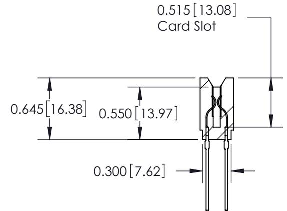
737 Series Ultra-Mate Card Edge Connector - Press Fit
