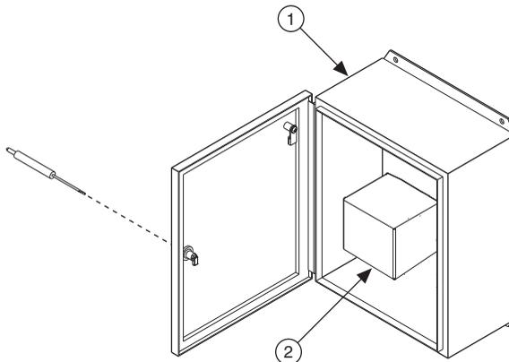
1 Suitably rated NEMA or IP enclosure that requires tool access
