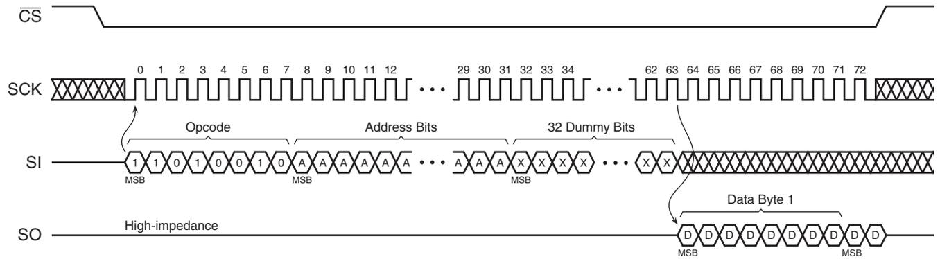
**Figure 25-5. Buffer Read (Opcode D4h)**
