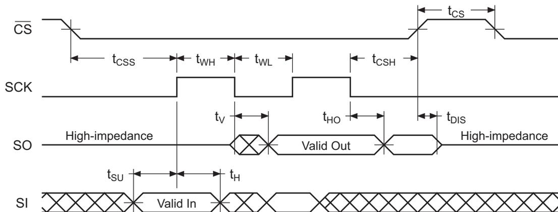
**Figure 22-2. Waveform 2 = SPI Mode 3 Compatible**
