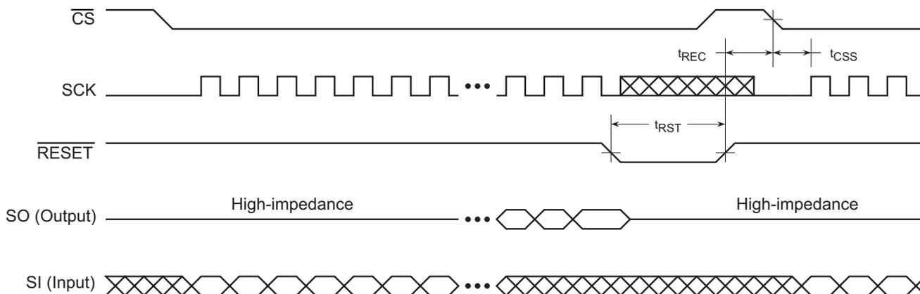
Note: 1. The  $\overline{CS}$  signal should be in the high state before the  $\overline{RESET}$  signal is deasserted.
