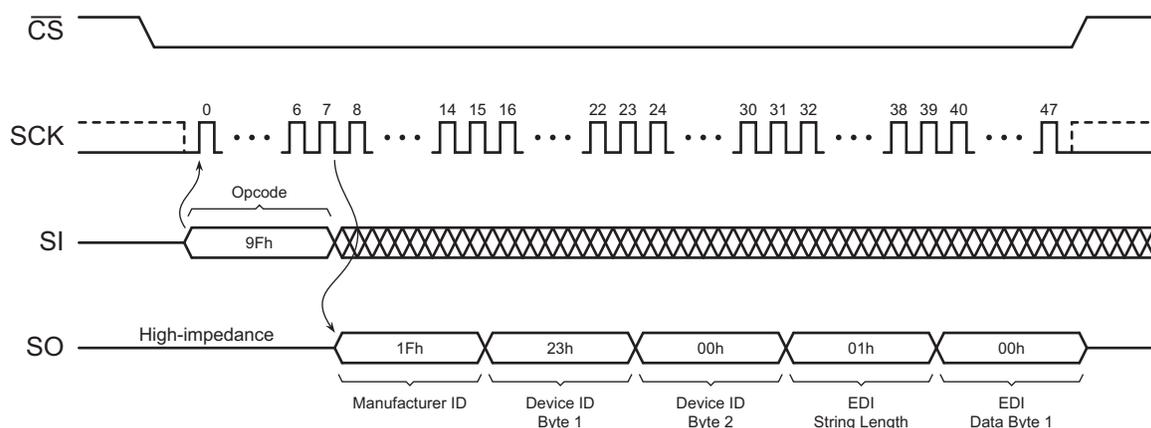
Note: Each transition
