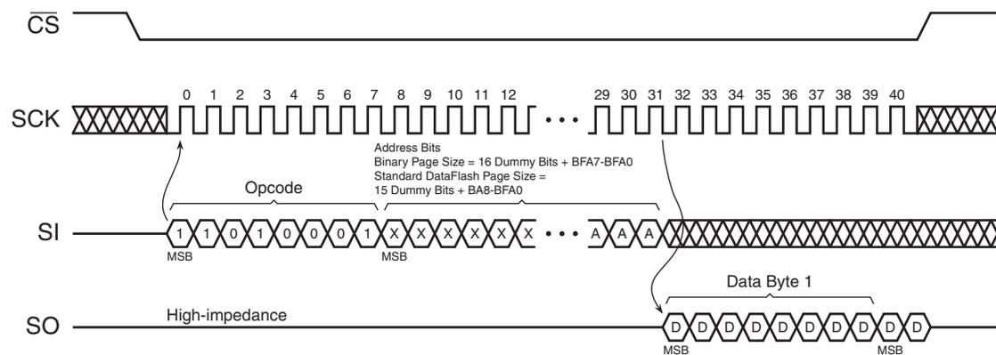
**Figure 25-7. Read Sector Protection Register (Opcode 32h)**
