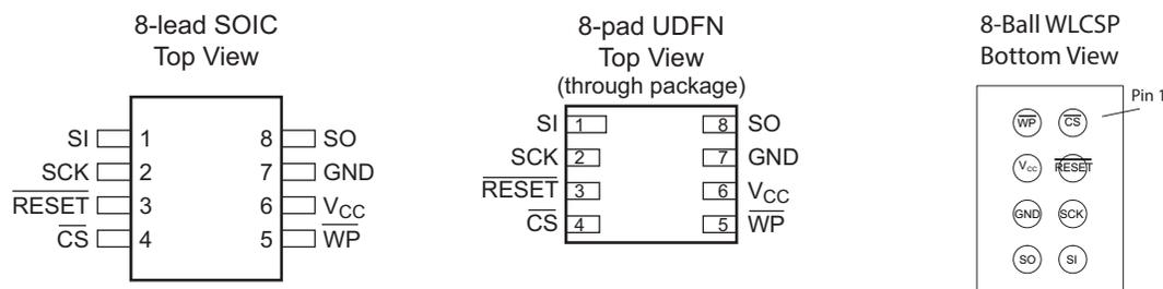
Note: 1. The metal pad on the bottom of the UDFN package is not internally connected to a voltage potential. This pad can be a “no connect” or connected to GND.
