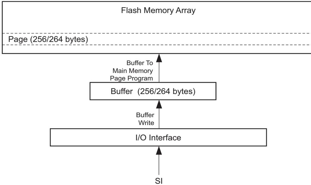
Figure 23-2. Buffer Write
