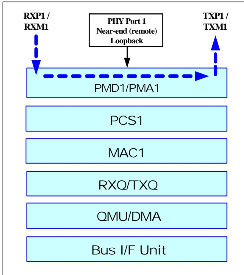
Figure 12. PHY Port 1 Near-end (Remote) Loopback Path
