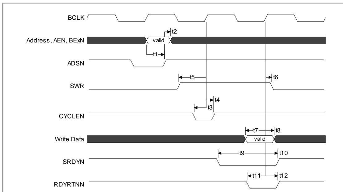
**Figure 19. Synchronous Write Cycle – VLBUSN = 0**
