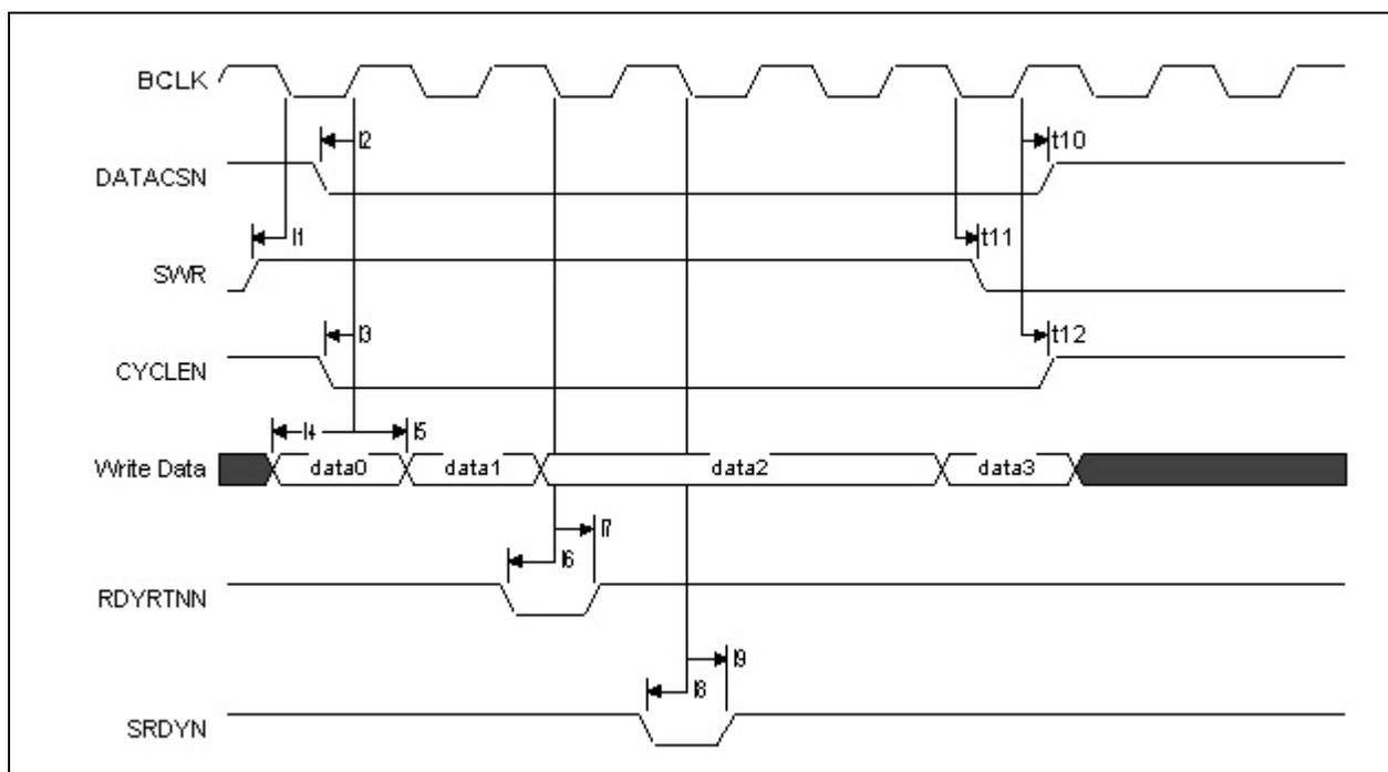
**Figure 17. Synchronous Burst Write Cycles – VLBUSN = 1**
