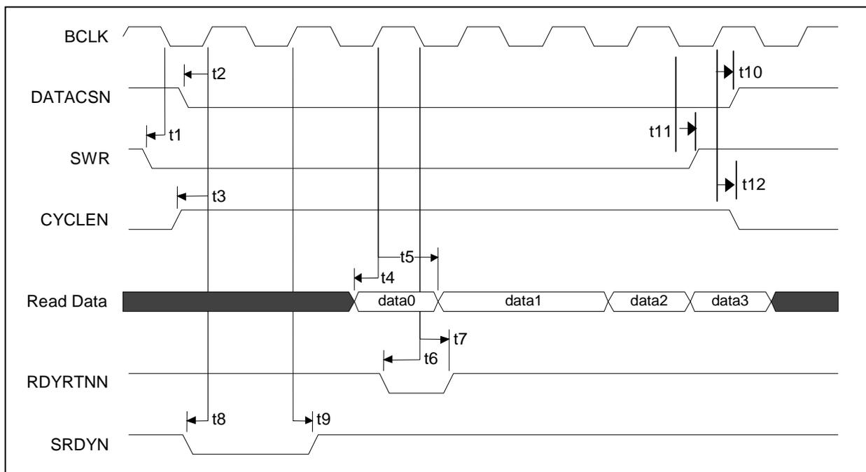
**Figure 18. Synchronous Burst Read Cycles – VLBUSN = 1**
