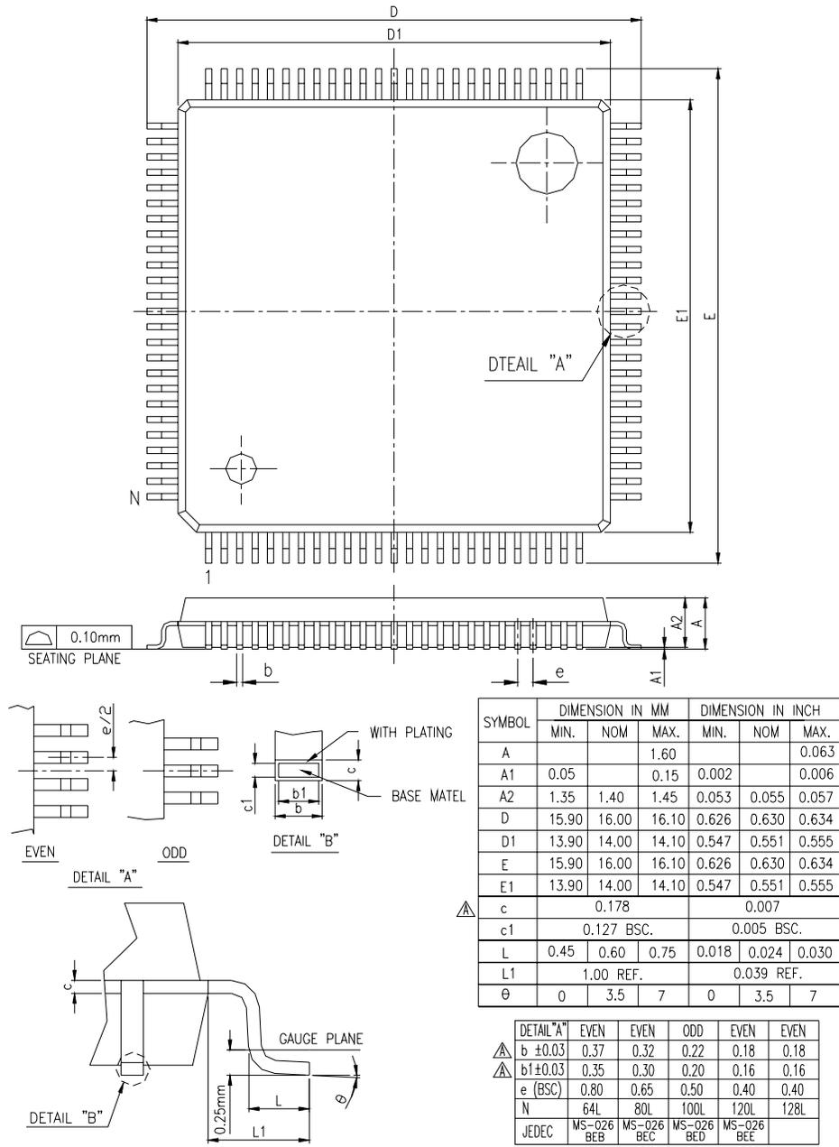
Figure 25. Optional 128-Pin LQFP Package
