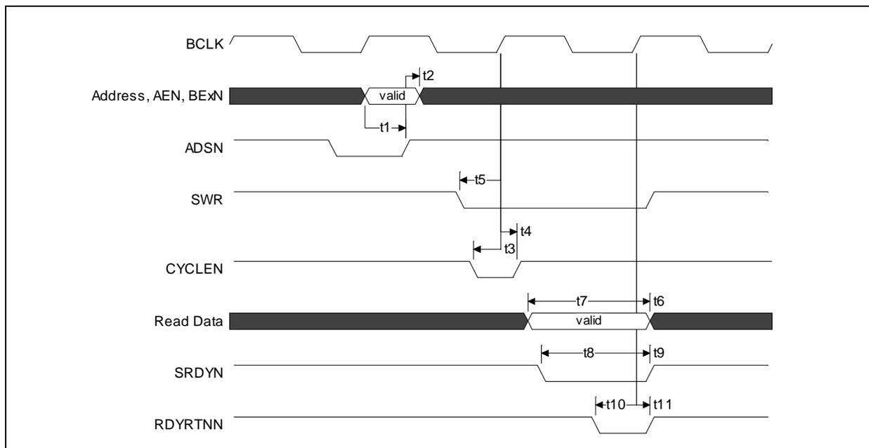
**Figure 20. Synchronous Read Cycle – VLBUSN = 0**
