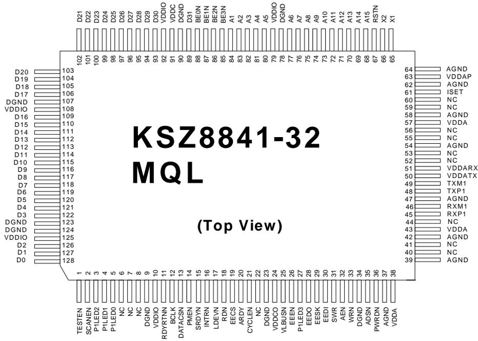
Figure 5. Standard – KSZ8841-32MQL 128-Pin PQFP
