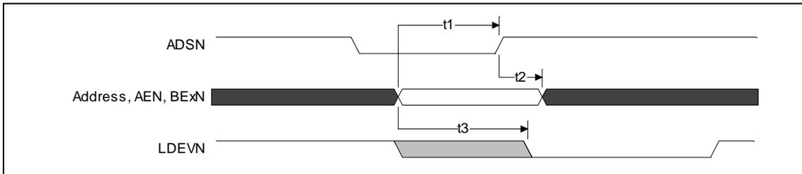
**Figure 16. Address Latching Cycle for All Modes**
