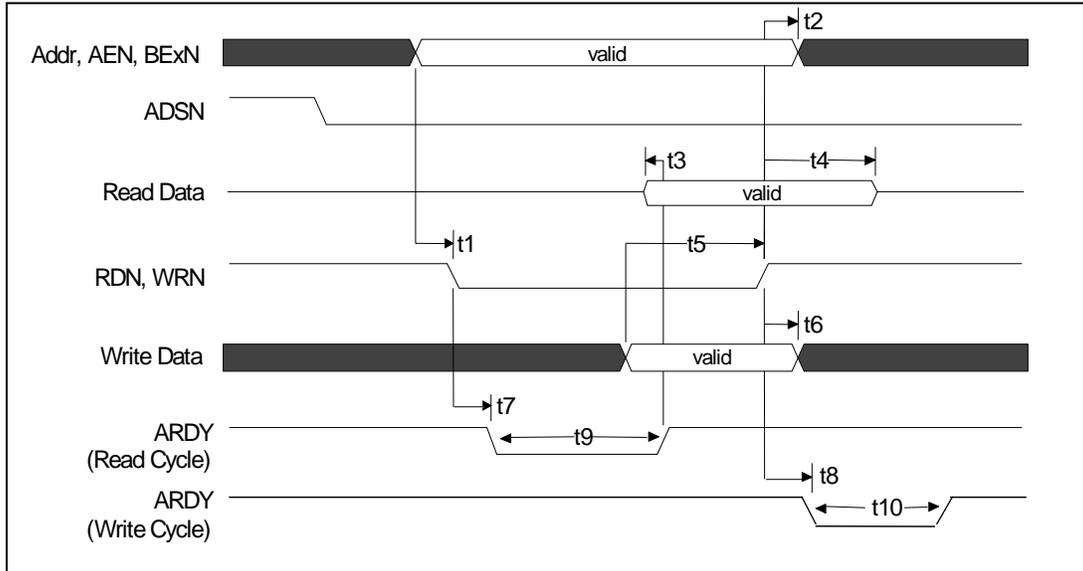
Figure 13. Asynchronous Cycle – ADSN = 0
